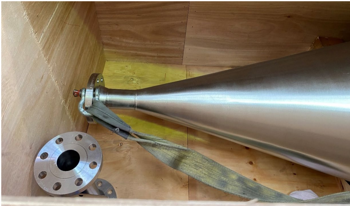
Figure 51. View of Outlet Flange and Trap for Particle Collection
