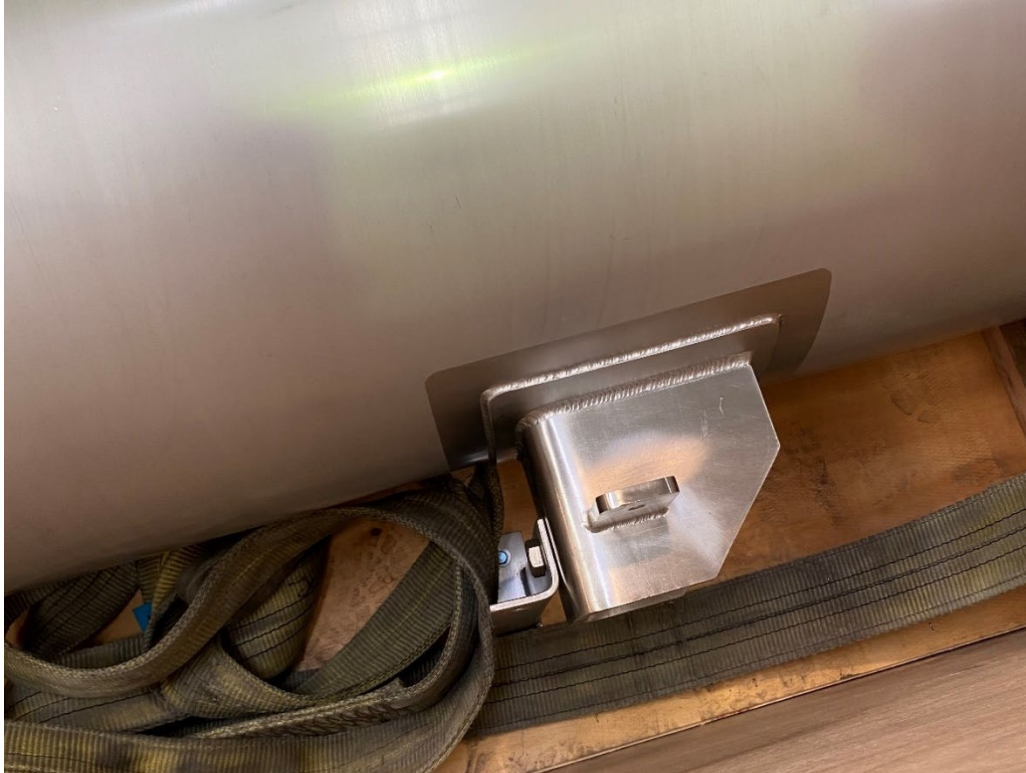
Figure 50. View of Support Bracket for Particle Separator Mounting
