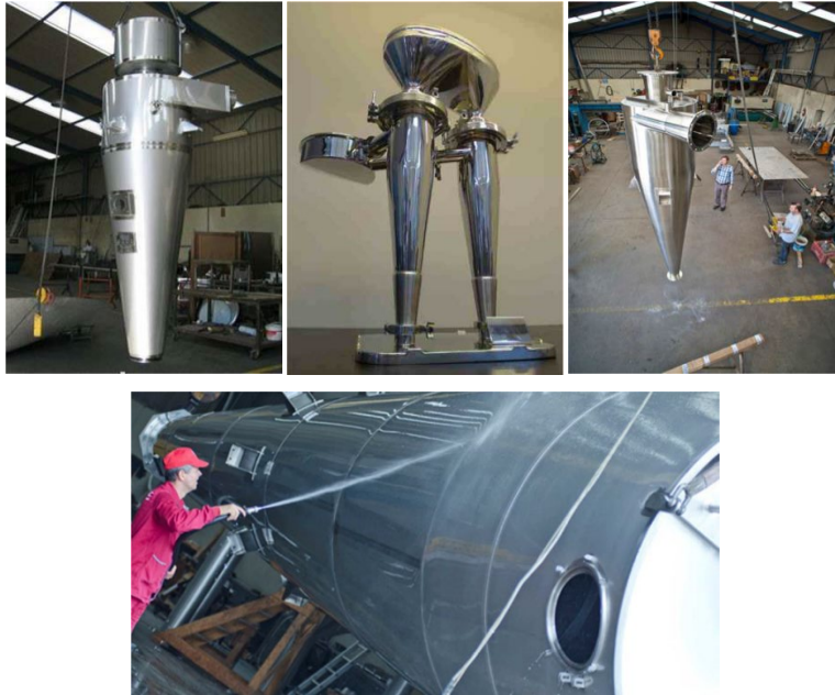
Figure 45 Pictures of Different ACS Cyclones
