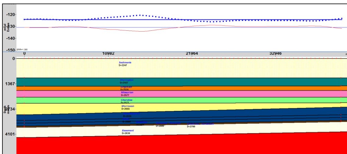
Figure 2.64: Model with basement depth 500 meters deeper results in a very small misfit ( \sim 1 mGal).
