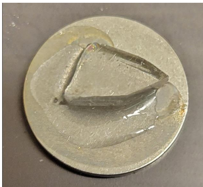
Figure S1: Example image of a barite crystal. The crystal is mounted on a 12 mm diameter AFM sample puck with Crystalbond™ 509 adhesive, with the fresh-cleaved 001 face exposed. Photo taken after experiment was complete.
