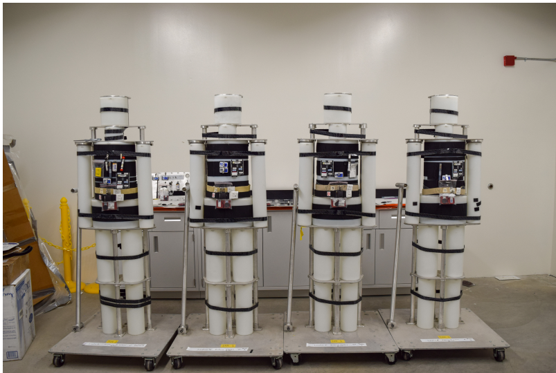
Figure 3.1: Example of four BOMABs assembled on stands with dosimeters placed on the front.
