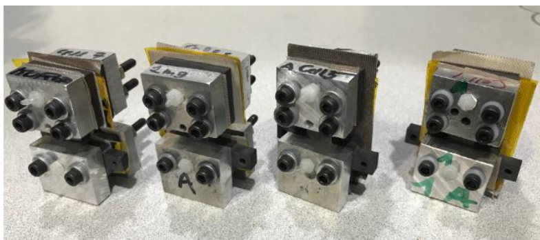
Figure 8. Photograph of assembled 4 electrolyzers that are ready for imaging.
