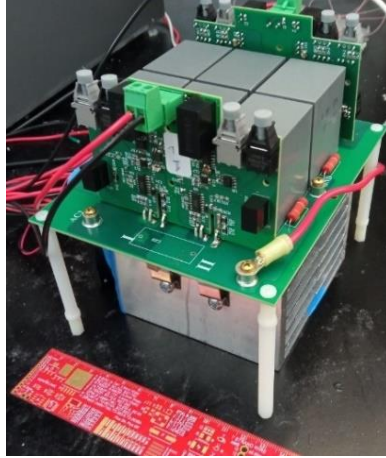
Fig. 2-41. Photograph of LV power stage
