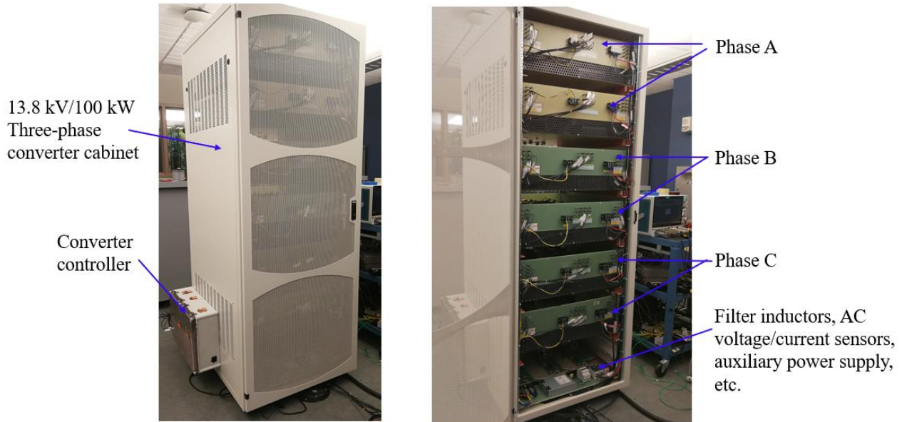
Fig. 2-15 Picture of the three-phase 13.8 kV/ 100 kW PCS converter
