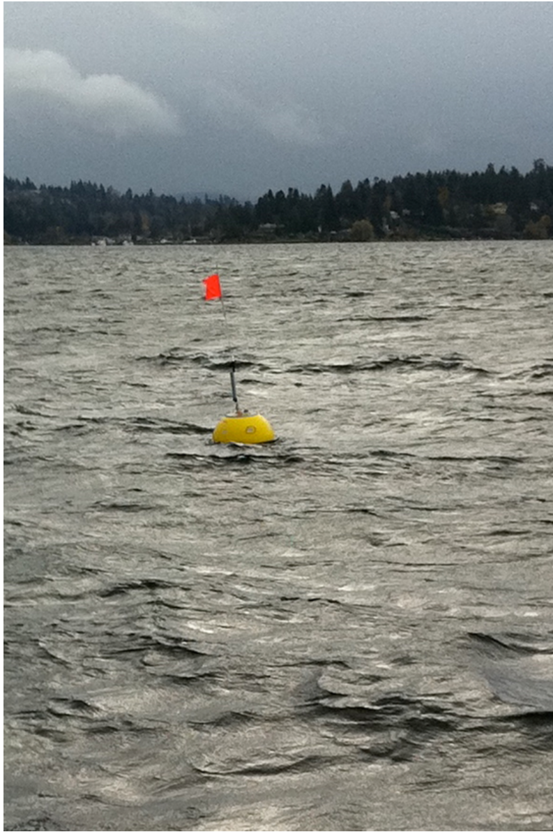
Figure 62: Waverider buoy deployed by the University of Washington located less than 1 km from the test site.
