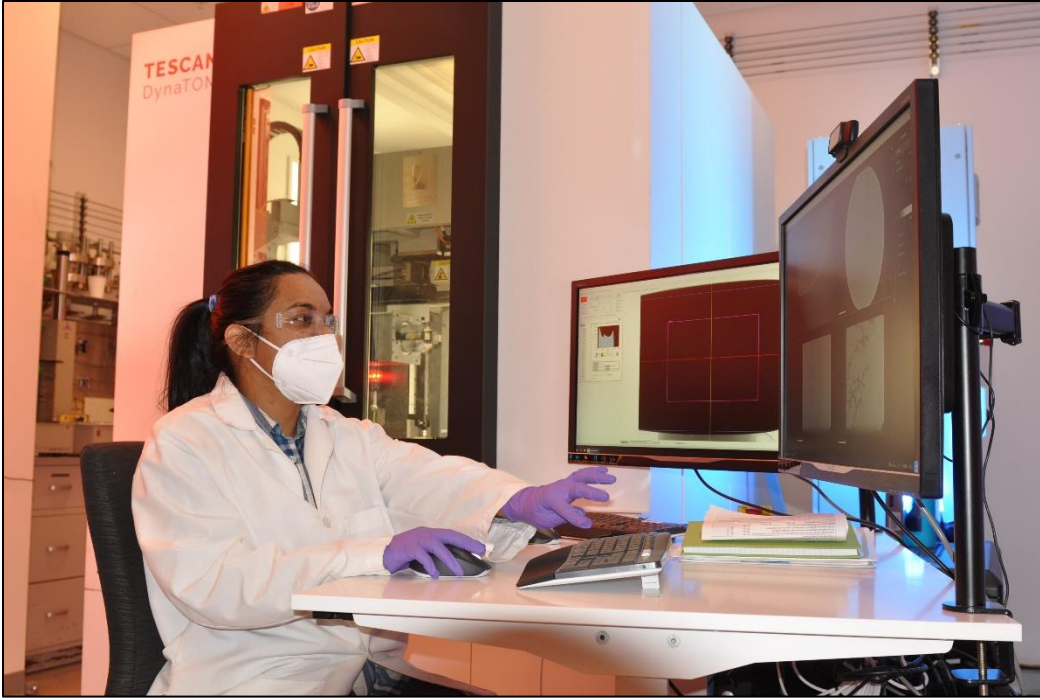
Figure 10: Tescan DynaTOM micro-CT scanner used for high-resolution CT images at NETL used for core analysis.
