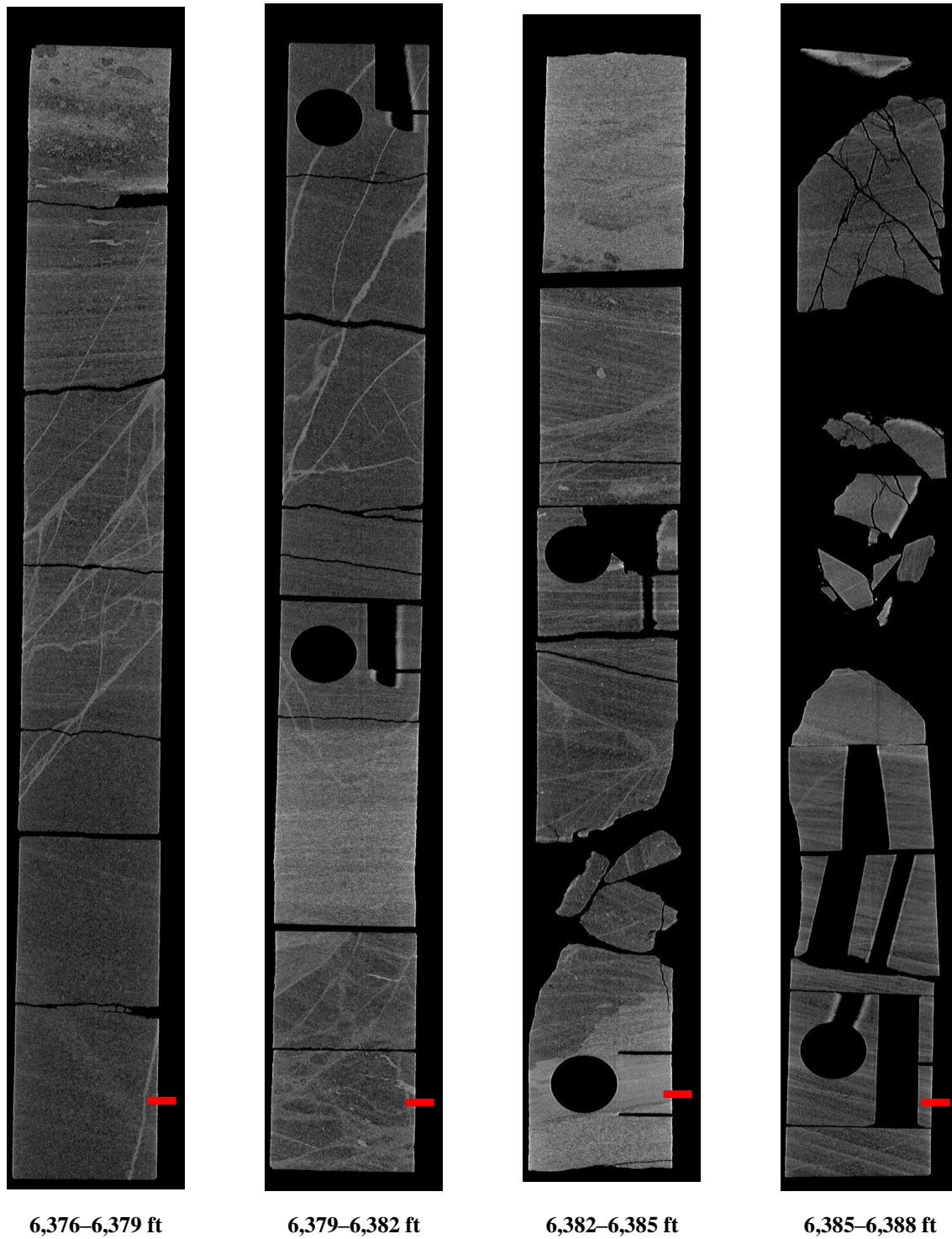
Figure 21: 2D midplanes of the medical CT scans of the OEE Well #1 from 6,376–6,388 ft.
