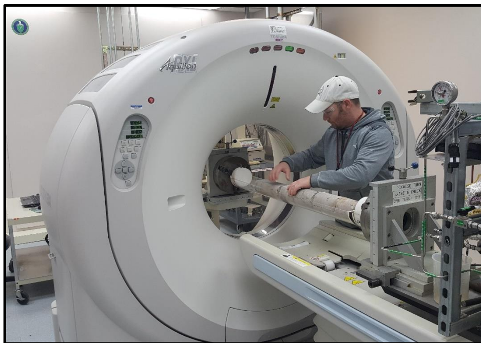
Figure 8: Toshiba® Aquilion™ Multislice Helical CT Scanner at the NETL used for core analysis.
