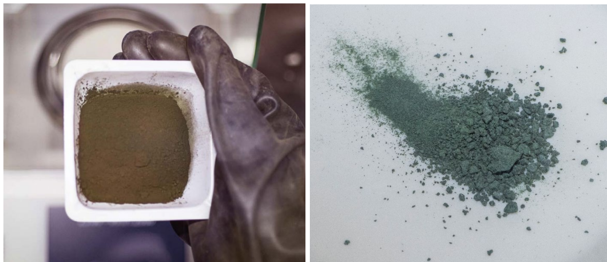
Figure 1: Photographs of ( left ) UCl 3 received from Terrapower, and ( right ) NaCl + 36 mol % PuCl 3 eutectic salt received from Idaho National Laboratory.
