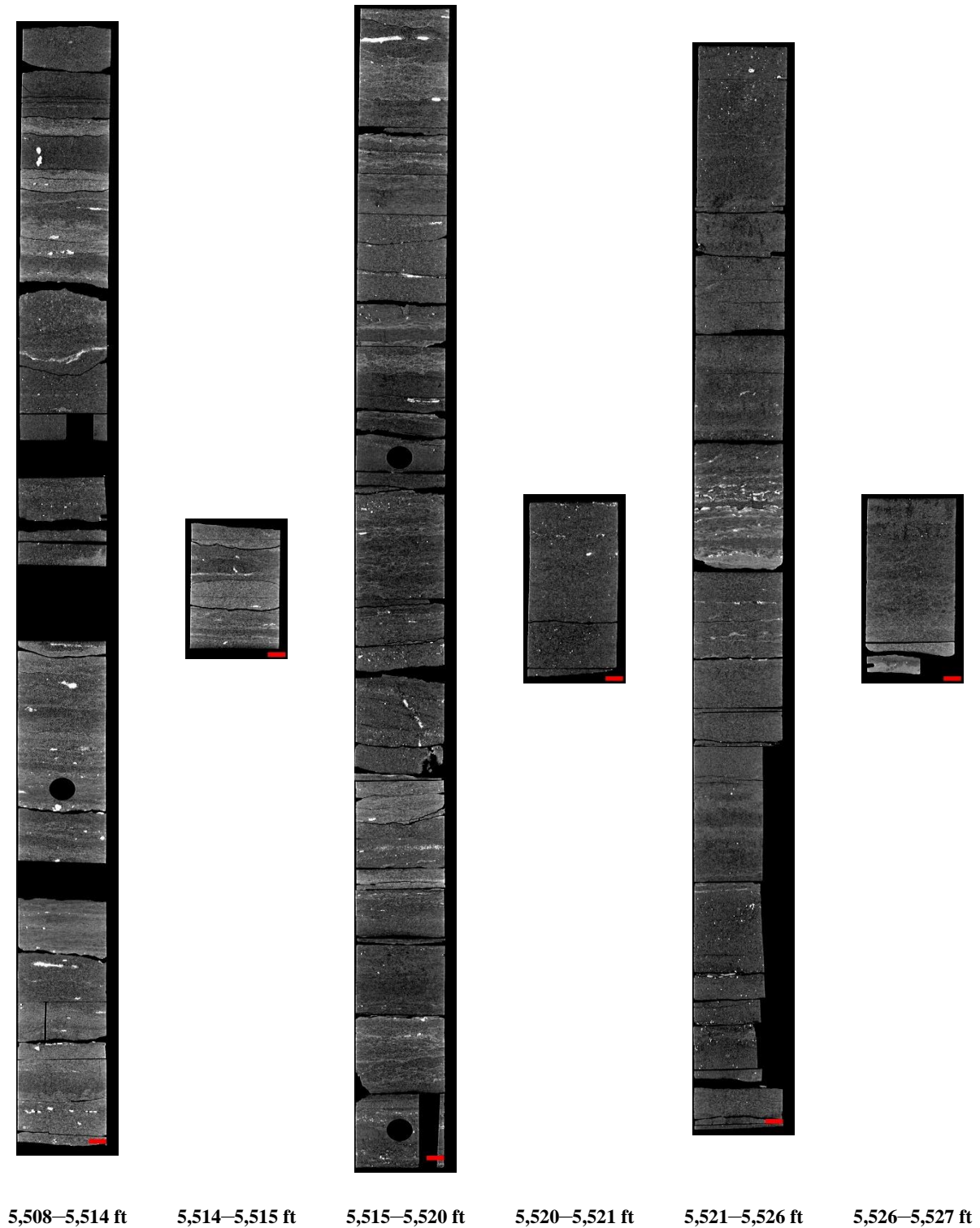
Figure 30: 2D isolated planes through the vertical center of the medical CT scans of the VW #1 well from 5,508 to 5,527 ft.
