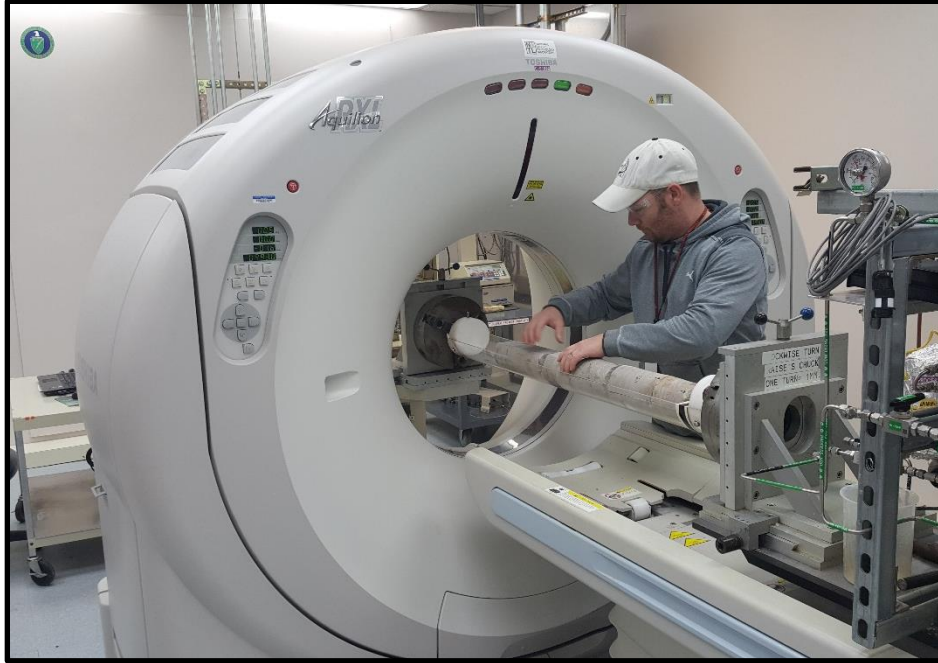
Figure 19: Toshiba® Aquilion™ Multislice Helical CT Scanner at NETL used for core analysis.
