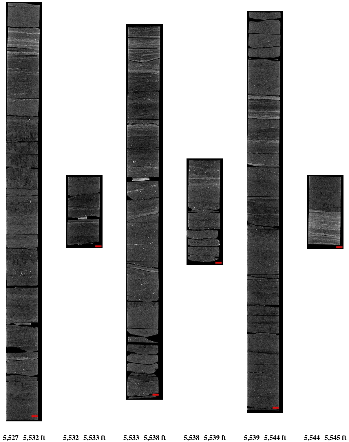
Figure 31: 2D isolated planes through the vertical center of the medical CT scans of the VW #1 well from 5,527 to 5,545 ft.
