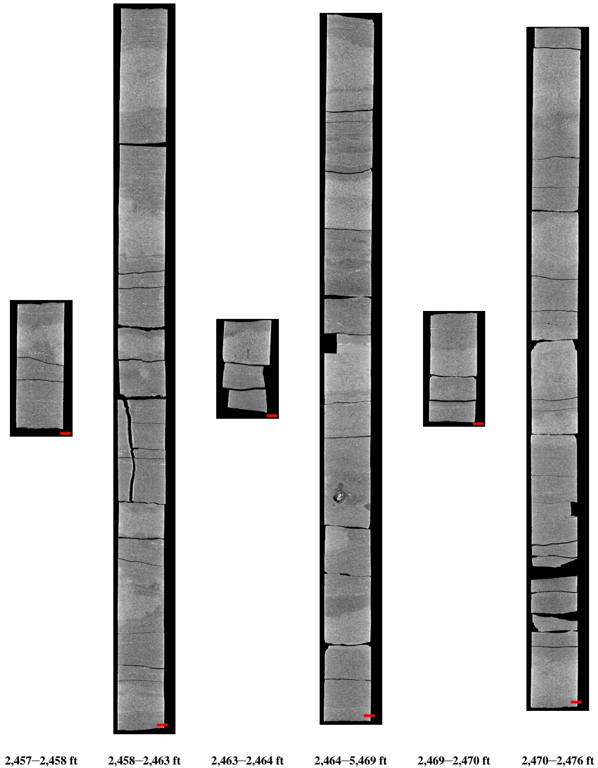
Figure 34: 2D isolated planes through the vertical center of the medical CT scans of the Wabash #1 well from 2,457 to 2,476 ft.
