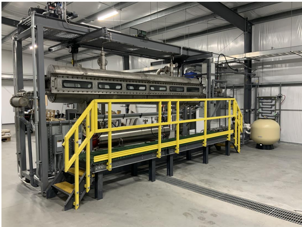
Figure 2-1 Heat Transfer Loop, condenser side
