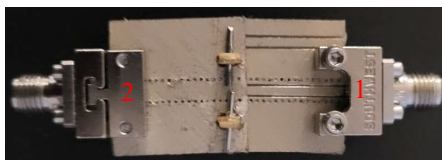
Figure 4. Fully assembled two-line (RF + DC) PEEK printed connector.
