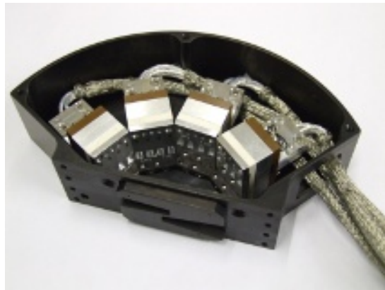
FIG. 2: Baffle-mounted bolometer camera, before installation. There are two apertures, each viewed by 2 4-channel sensors. A plate (not shown) sits between the apertures and sensors to prevent light from the wrong aperture reaching the sensor. The plate is ridged, and all the internal surfaces of the camera and blackened, to reduce internal reflections.
