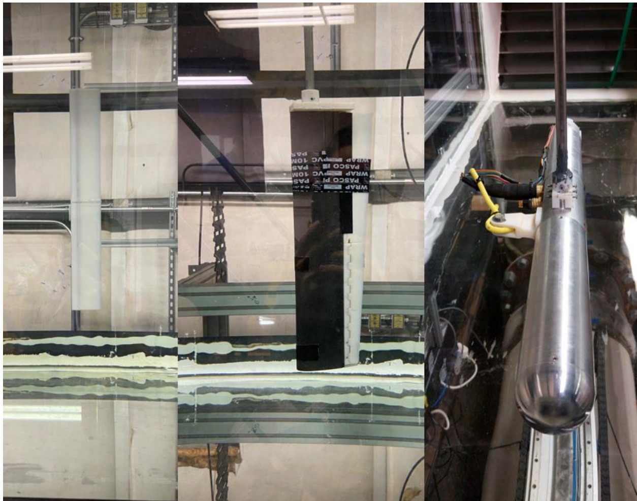
Figure 41: From left to right; the elevator, wing, and fuselage with tether components as vertically strut mounted in the water tunnel.
