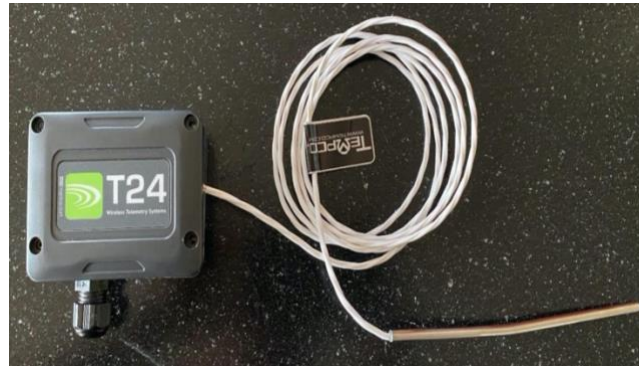
Figure 2.3: Image of transmission module connected with temperature sensor
