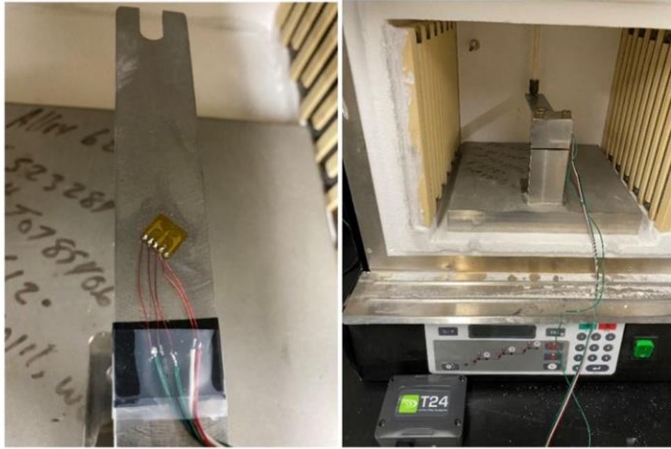
Figure 2.2: Image of the strain sensing setup integrated with an oven
