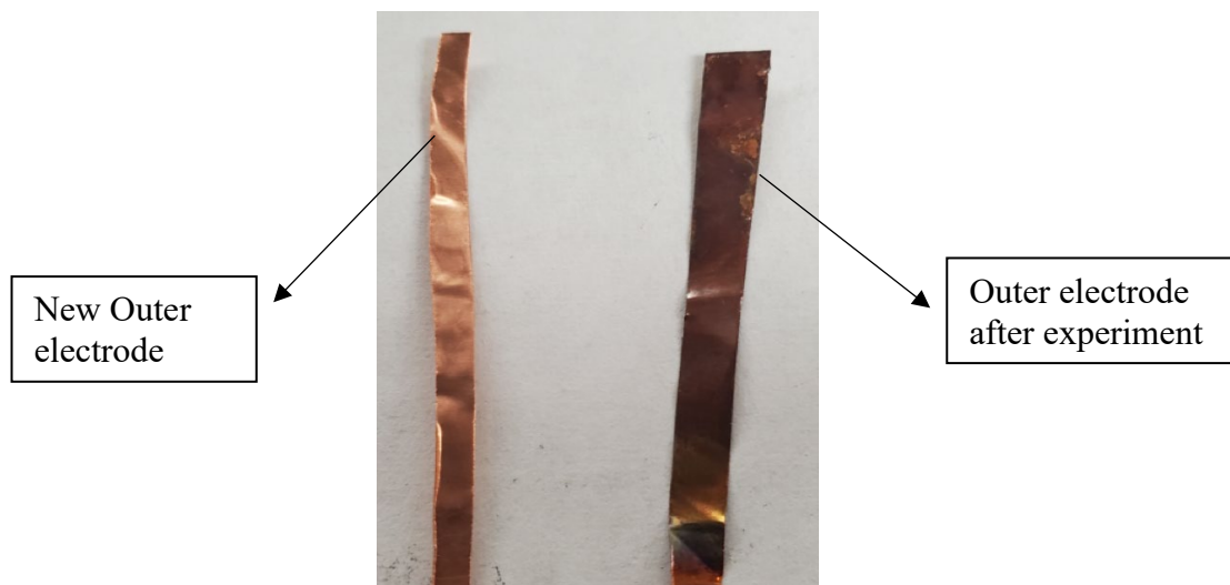
Fig. 3. Electrode comparison before and after experiments
