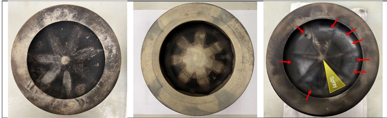
Figure 38: Tested TBC pistons in the SCTE showing soot deposits, successful coating adhesion, and coating delamination (right piston)
