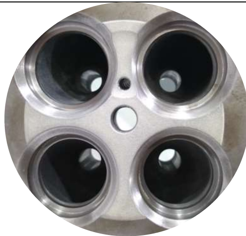
Figure 101: TBC Cylinder Head Successfully Manufactured
