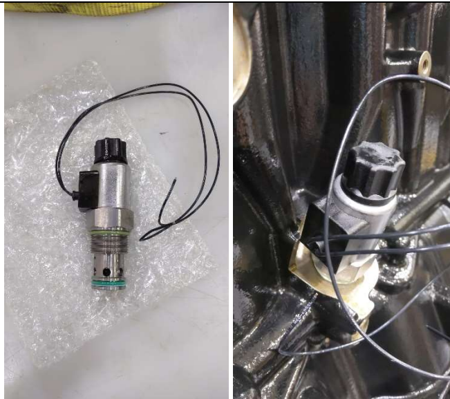
Figure 103: Solenoid unpackaged and installed into engine block
