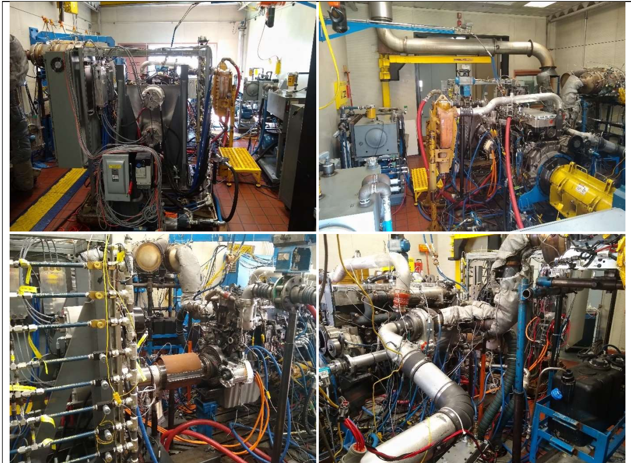
Figure 121: Final H2D2 Full Hybrid System validation test installation which included the 13L concept engine, SuperTurbo, emissions aftertreatment catalysts, 48V MGU and battery emulator, HSFW electric drive, hybrid oil and coolant supply units, and numerous testing support systems.
