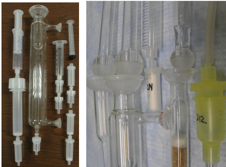
Fig. 3. Examples of attachable columns for requirements of volume, temperature and effluent loading.
