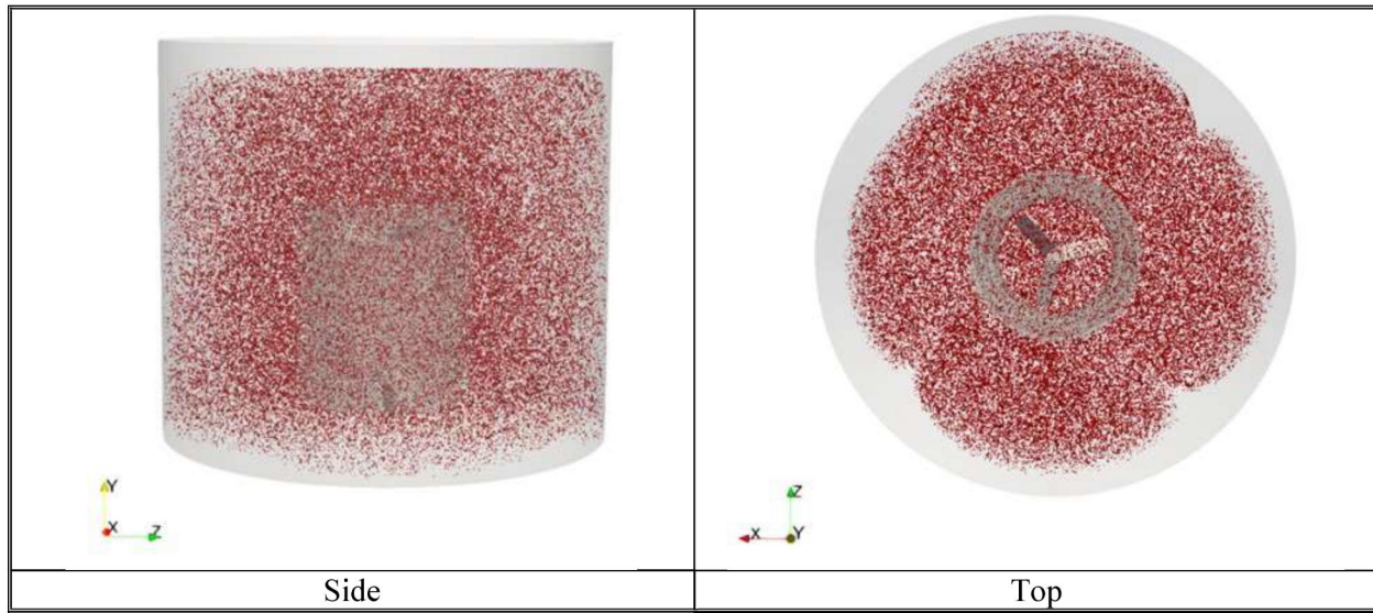
Figure 5. Dispersion of particles after Mixing for 60 seconds in the SME with 4 Blades on the Bottom Impeller
