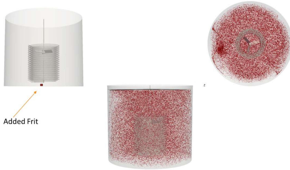
Figure 14. Dispersion of Added Glass Frit Particles after Mixing the SME for 300 Seconds
