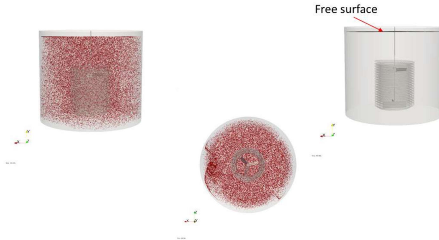
Figure 11. Dispersion of Particles after Mixing for 300 seconds in the SME with 3 Blades on the Bottom Impeller with a Free Surface
