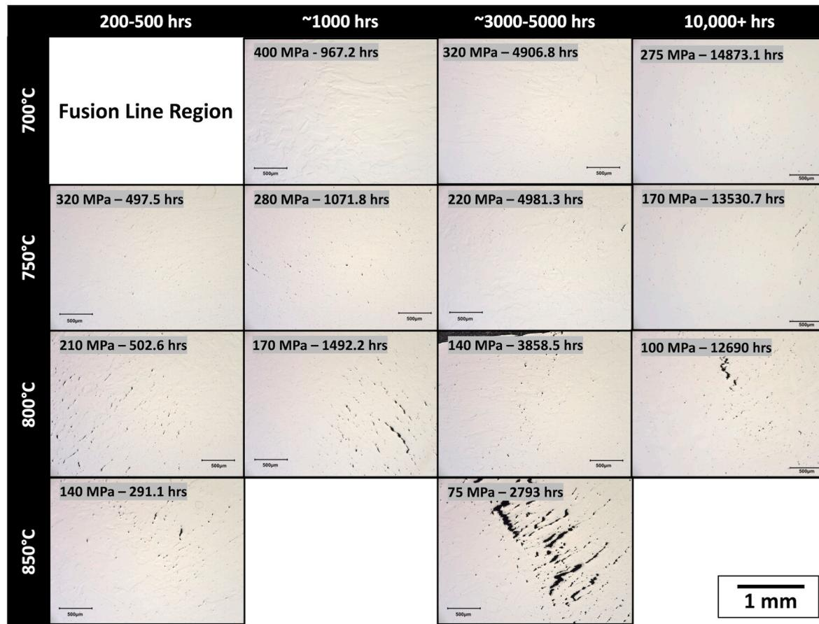
Fig. 7. Unetched micrographs of the FL regions including HAZ and WM after creep testing showing creep damage. Applied stress is in the horizontal axis.
