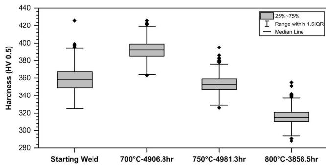
**Fig. 10.** Post-test base metal hardness distributions (see Fig. 9) with outliers (diamonds). The shaded boxes are defined by the upper and lower quartiles (25%–75%) which are the values halfway between the mean and largest or smallest value respectively, and the outliers are those values falling outside 1.5 times the inner quartile distance (Range within 1.5IQR).
