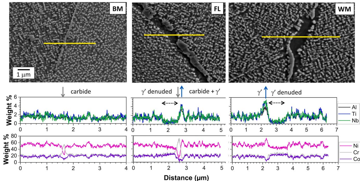
**Fig. 13.** BSE images with EDS line scans identifying grain boundary carbide formation and coarsened  $\gamma'$  associated with  $\gamma'$  denuded zones in FL and WM regions in contrast to the BM after creep testing at 750 °C for 4981.3 h. Down arrows indicate location of carbides, up arrows  $\gamma'$ , and double ended arrow  $\gamma'$  denuded regions.
