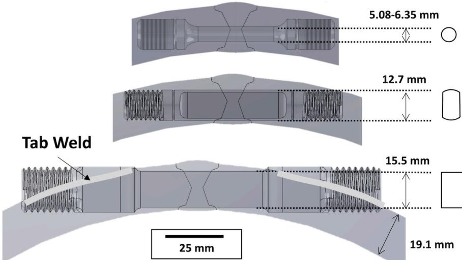
Fig. 2. Cross-weld creep sample designs.
