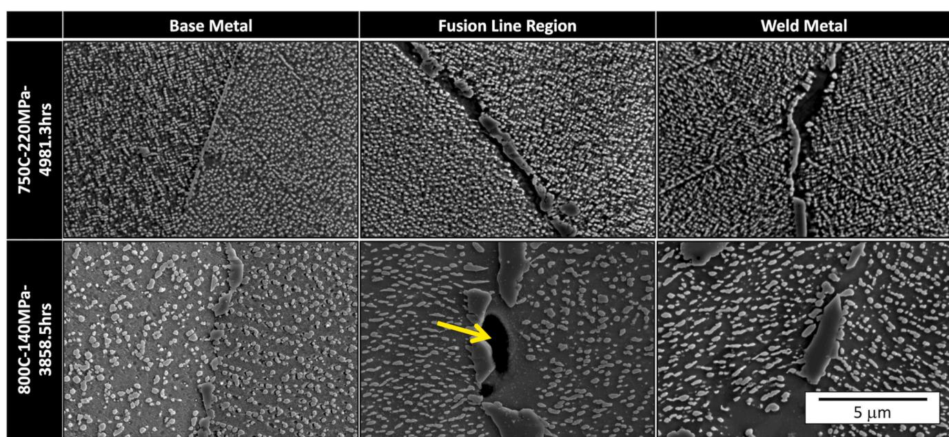
**Fig. 11.** BSE Images of grain boundaries in the BM, FL, and WM regions after creep testing. Applied stress is in the horizontal plane and the arrow indicates a creep void forming on a grain boundary normal to the applied stress.
