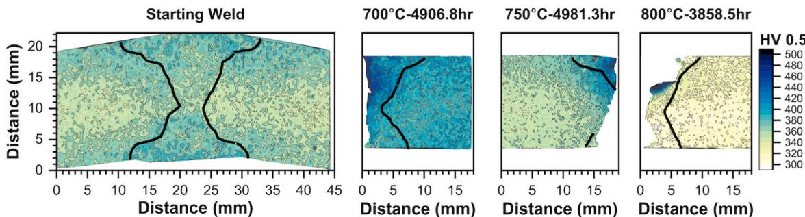
Fig. 9. Weldment hardness distribution for the starting weld and selected samples after creep exposure. Approximate location of the FL is indicated by the solid line for each sample.
