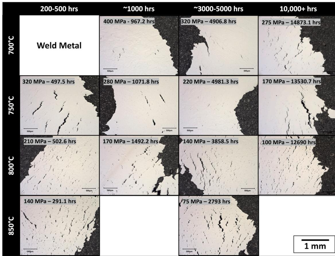
Fig. 8. Unetched micrographs of the WM after creep testing showing creep damage. Applied stress is in the horizontal axis.
