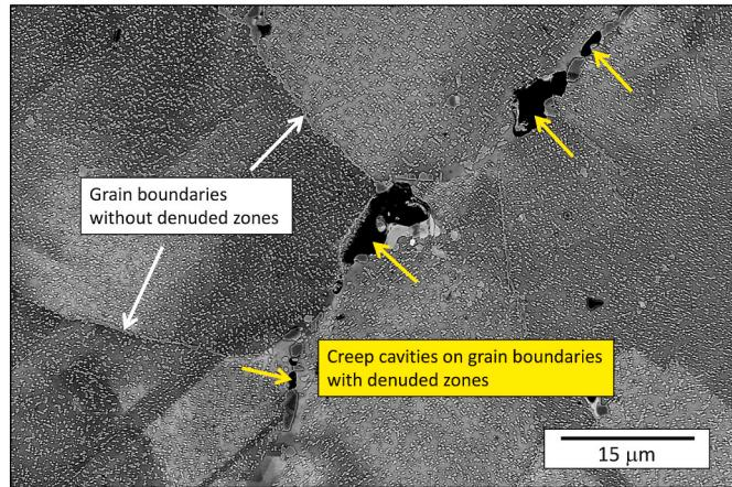
**Fig. 12.** Creep cavitation in the weld metal after testing at 800 °C for 3858.5hrs. Applied stress is in the horizontal plane.
