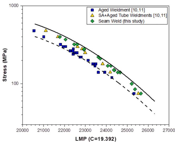
**Fig. 6.** LMP ( $C = 19.392$ ) plot for alloy 740H seam welds compared to average base metal (solid line) and 30% reduction on stress (dashed line). Data for previous research on weldments made with matching filler metal for both welded + aged (Aged Weldment) and welded + solution annealed + aged (SA + Aged Tube Weldments) are included for comparison [10,11].
