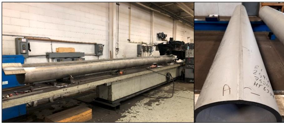
Fig. 1. Pipe during fabrication (left) and finished pipe (right).
