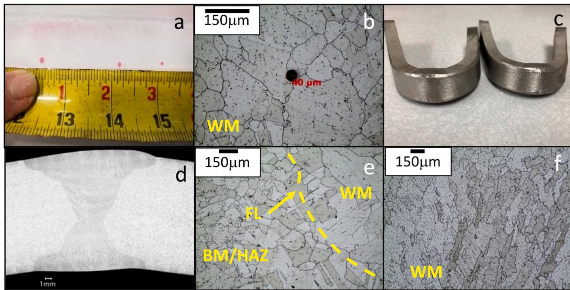
**Fig. 3.** Isolated non-rejectable surface (a) and WM (b) porosity (40  $\mu\text{m}$  diameter pore indicated); example of successful bend tests (c); macro showing overall weld geometry and structure (d), and representative micrographs of the FL region (e) and WM (f) showing recrystallization and no evidence of microfissures, LOF, cracking or other weld defects.
