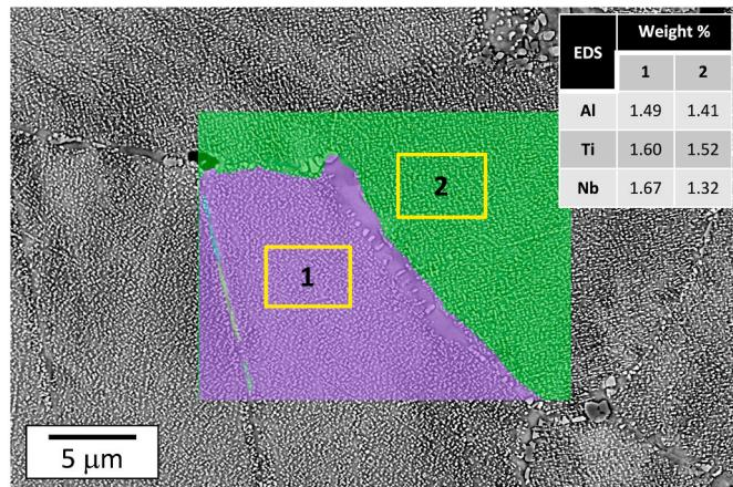
**Fig. 15.** EBSD orientation map overlayed on BSE image of an alloy 740H grain boundary after creep testing with inlaid EDS area spectrum for two grain interiors.
