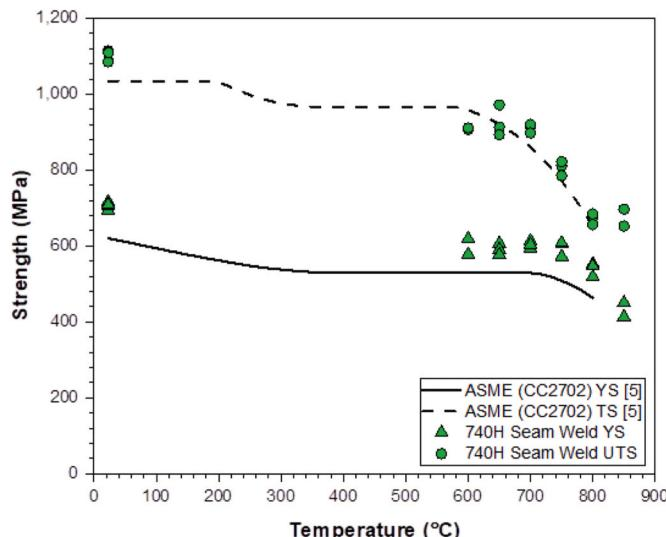
**Fig. 4.** Tensile test results for the alloy 740H seam weld.
