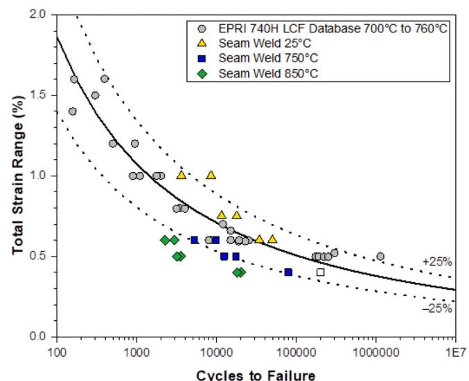
**Fig. 5.** LCF test results for alloy 740H cross-weld samples tested at room temperature (triangles), 750  $^{\circ}\text{C}$  (squares), and 850  $^{\circ}\text{C}$  (diamonds) compared to the EPRI wrought 740H LCF database (circles) which is combination of data from Refs. [33,34,36,37], open symbols represent tests which were stopped prior to failure (run-out condition).
