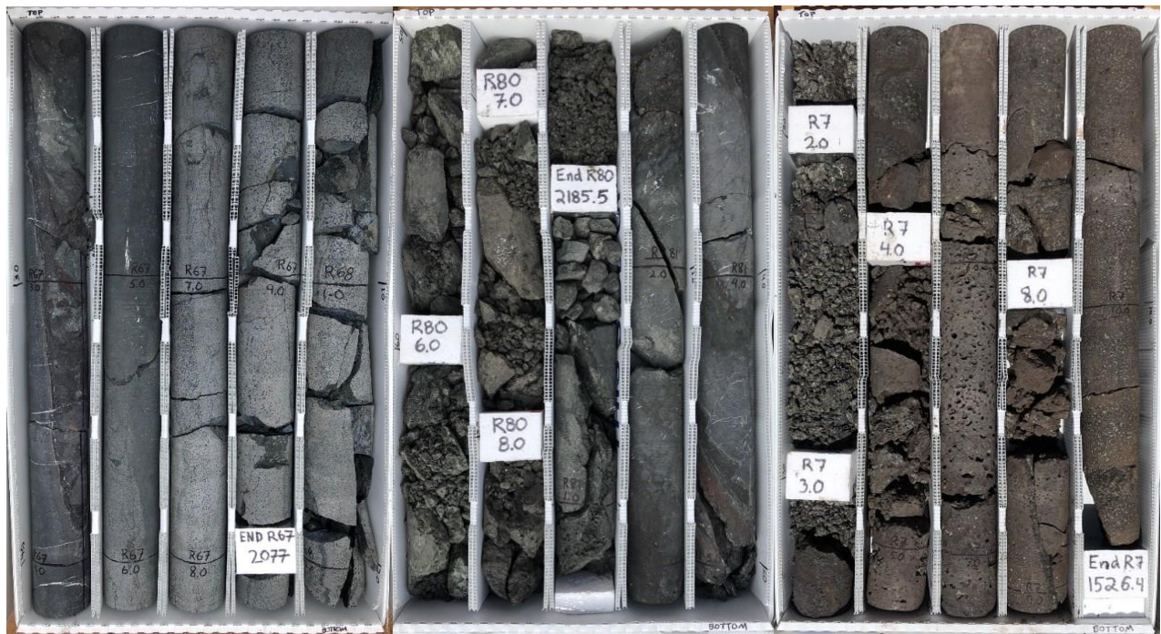
Figure 18. Cleaned, cut, and boxed rock core recovered from Lāna‘i Well 10. (Left) Example of solid, consolidated units within the borehole Evidence of a high-angle dike intrusion into the surrounding rock (left-most column in the core box). (Center, Right) Example of friable formations downhole. Most of this material came out of the core tube in a fairly competent form but clearly broke apart as they dried. This was milled up in between the drill string and the borehole walls into a fine sand.
