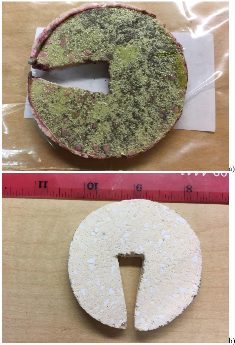
Figure 3.3. Photographs of interior side of Zirmul cover a) after Stage Two K-3 corrosion experiment (Test LA20-2c2), and b) clean Zirmul cover before corrosion experiment.
