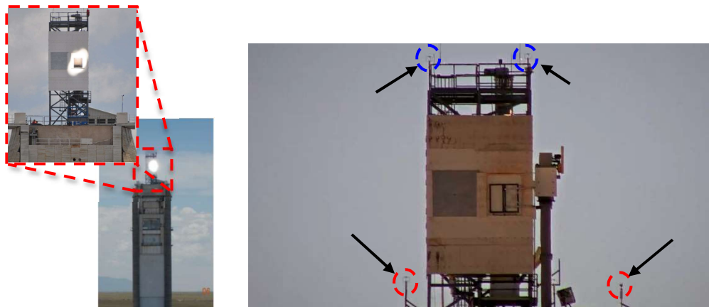
FIGURE 1. Receiver module atop the 61 m solar tower during an experiment (left) with 3D anemometers placed around the receiver module (right). Anemometers at the top of the receiver module (blue) measured free-stream velocity, and anemometers below the module (red) were used for validation.
