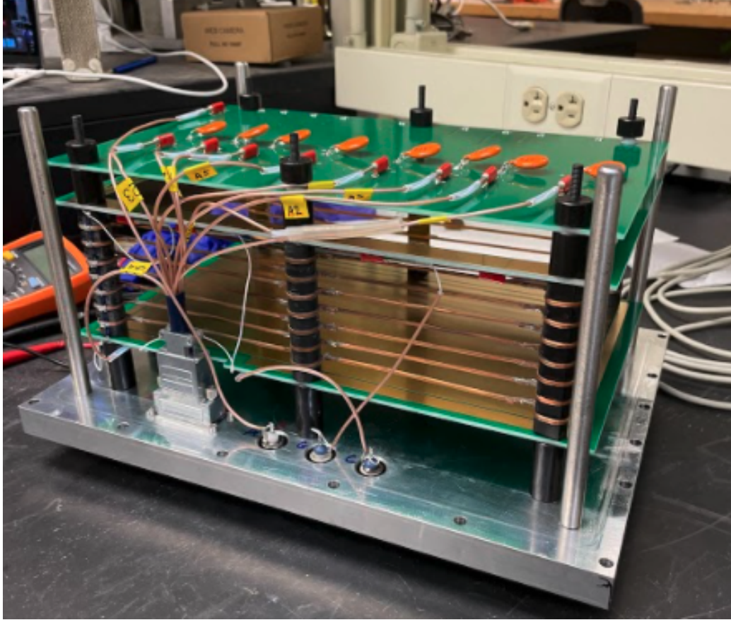
Figure 3: The top plate of the MONICA detector inverted on a tabletop, with the internal fixtures attached. The green plates are the cathode, Frisch grid, and anode from bottom to top and field cage electrodes surrounding the sides.
