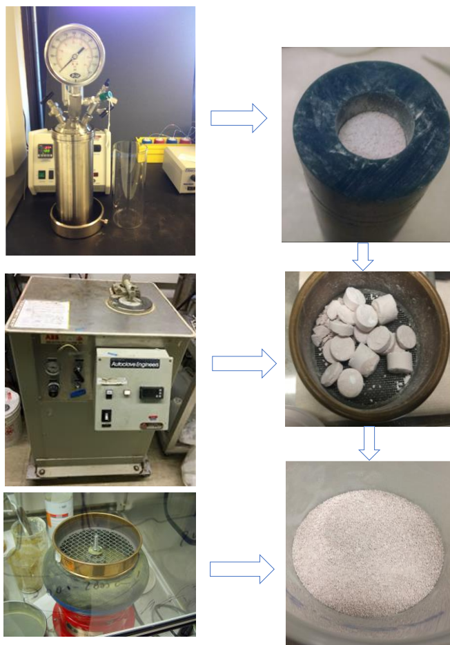
Figure 3. Two-liter Parr reactor and isostatic press used to fabricate the synthesized MOF powder into engineered particles.
