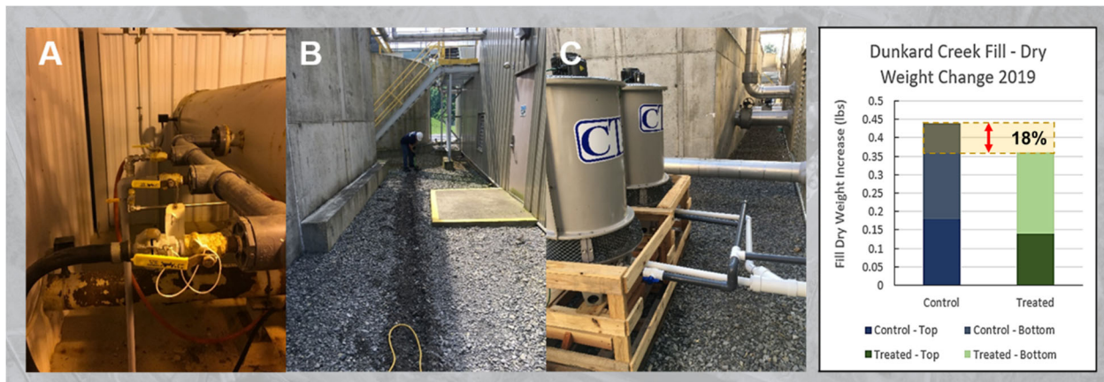
Figure 8. THERMOPHASE Cooling Tower Fill Reduction. THERMOPHASE treatment reduced dry weight by 18%. Small-scale cooling towers installed at water treatment station, circulating raw untreated water over the 2019 fouling season. Towers treated with Interphase technology showed increased fouling resistance, accumulating 18% less dry weight fouling.
