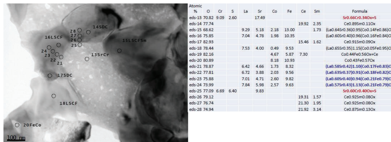
Figure 8 Typical chemistry of the LSCF and SDC grains next to the SrCrOx that are accumulated in the original pore regions.
