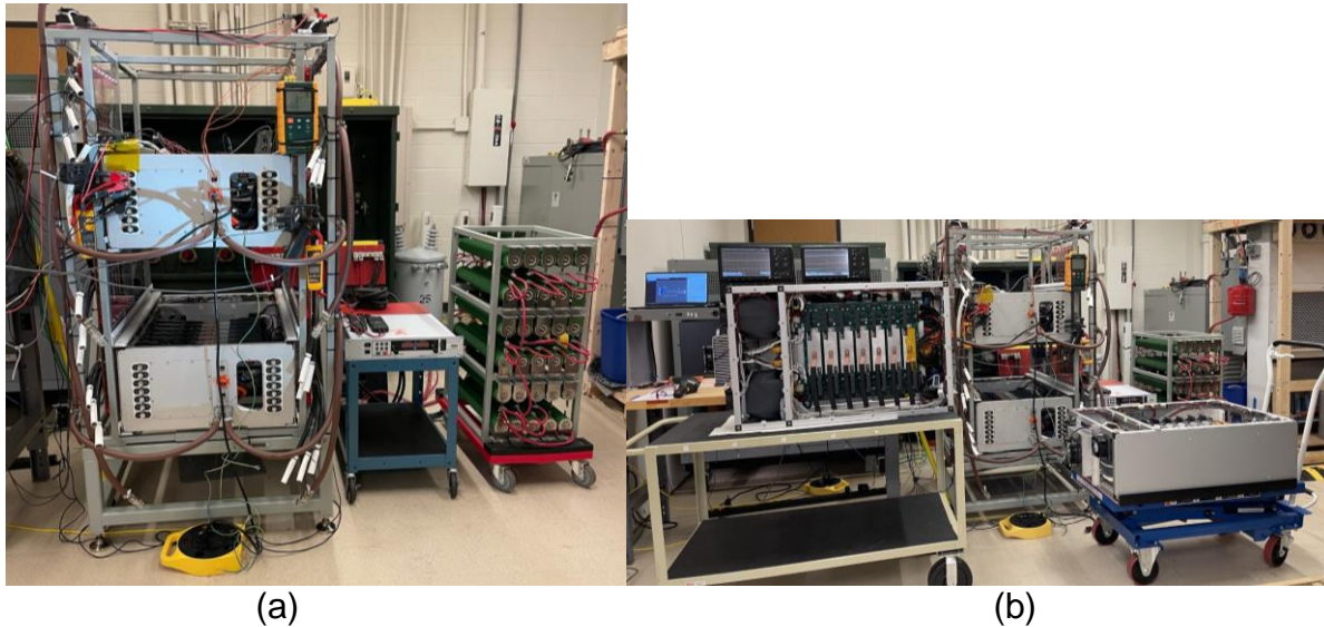
Figure 55: MDCT testing. (a) Two 75 kVA MDCT trays operating in parallel. (b) Four MDCT trays built complete.
