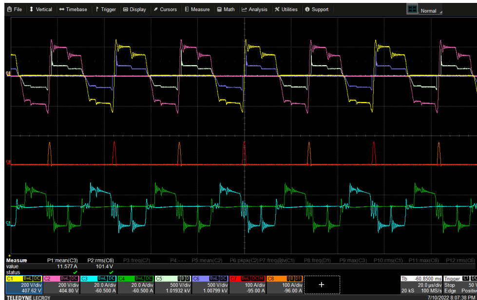
Figure 56: MDCT testing — two 75 kVA MDCT trays operating in parallel.
