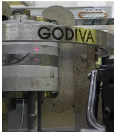
Visible PVD Probes During Setup on Godiva Assembly
