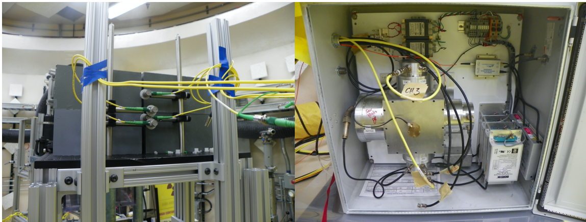
The PDV probes and internal view of the MHD-240 detector.
