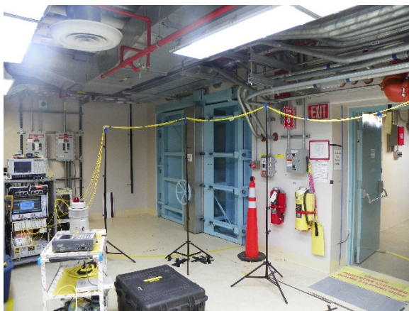
PDV Laser, scopes and associated equipment
