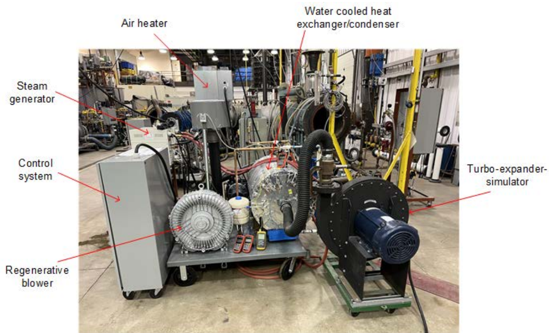
Figure 18. Assembled PDHS prototype test bench
