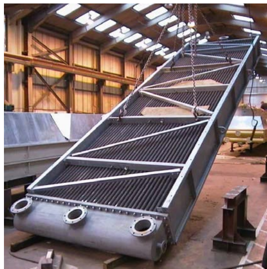
Figure 32. An air-to-water heat exchanger unit (HMX)
