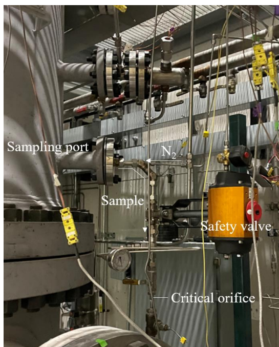
Figure 179. Ash aerosol sampling system mounted on BYU reactor
