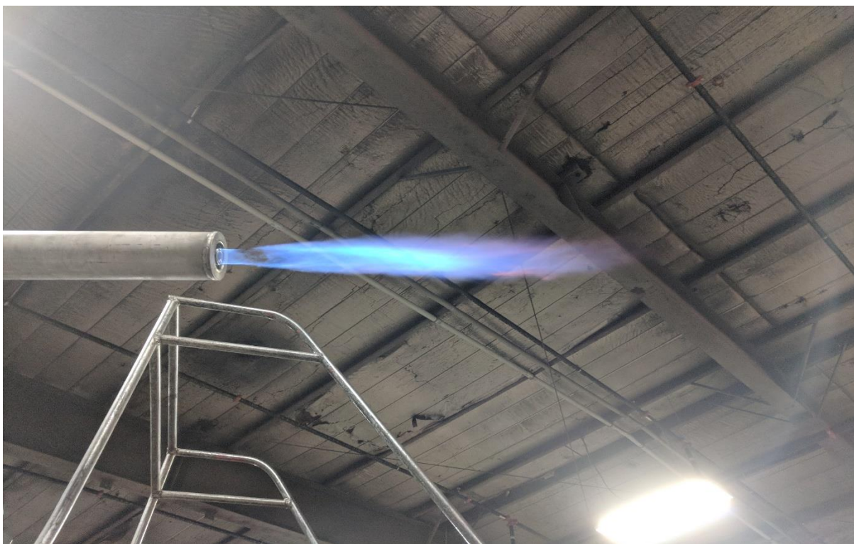
Figure 96. Ex situ burner flame calibration on natural gas
