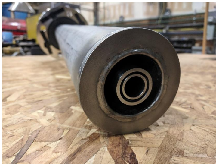
Figure 95. Photograph of the burner registers and water jacket
