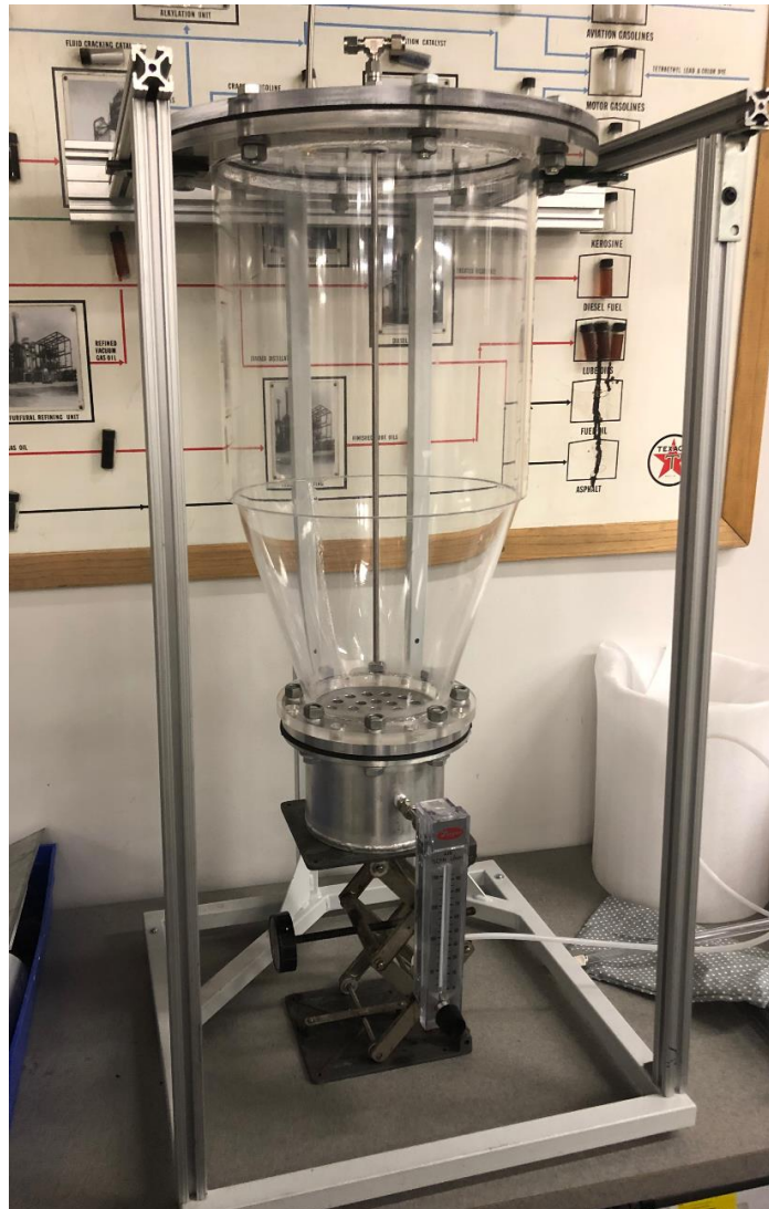
Figure 17. Acrylic cold-flow model of dry feed system hopper
