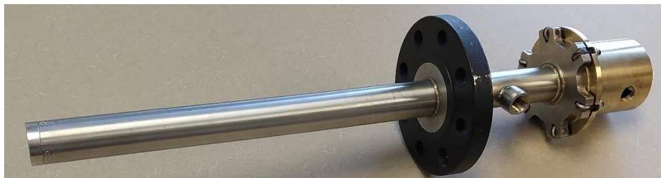
Figure 184. Image of completed high-pressure corrosion probe body built at BYU's Precision Machine Shop
