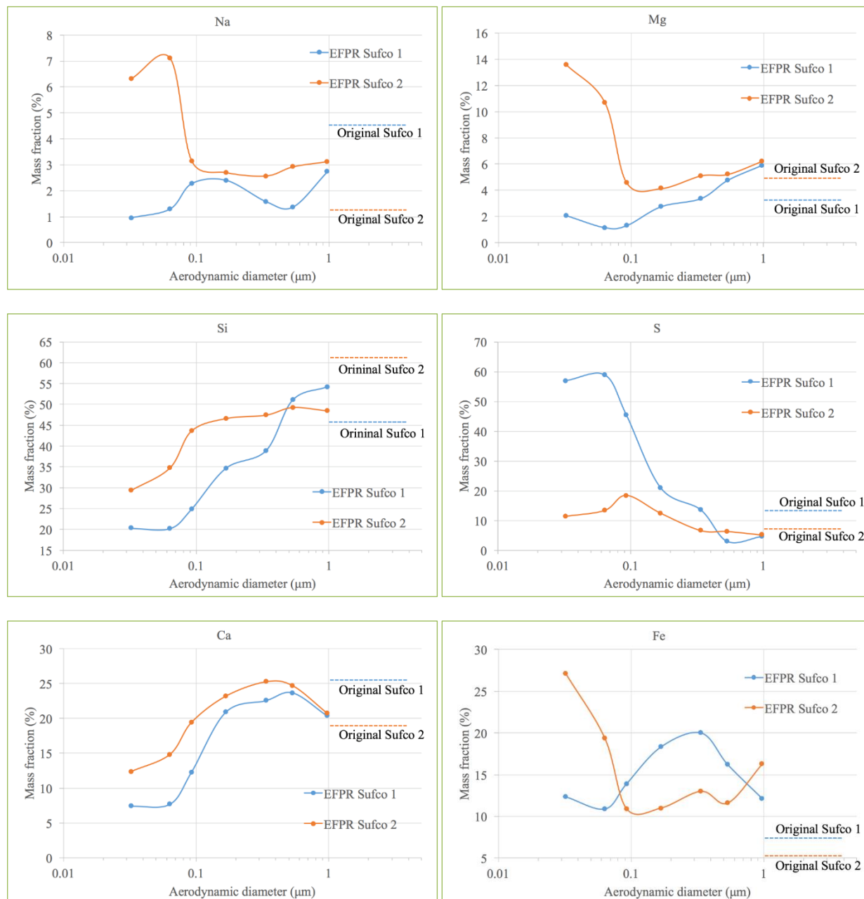
Figure 154. Composition of size-segregated ash aerosol in EFPR (BLPI: 1-7 stages)
