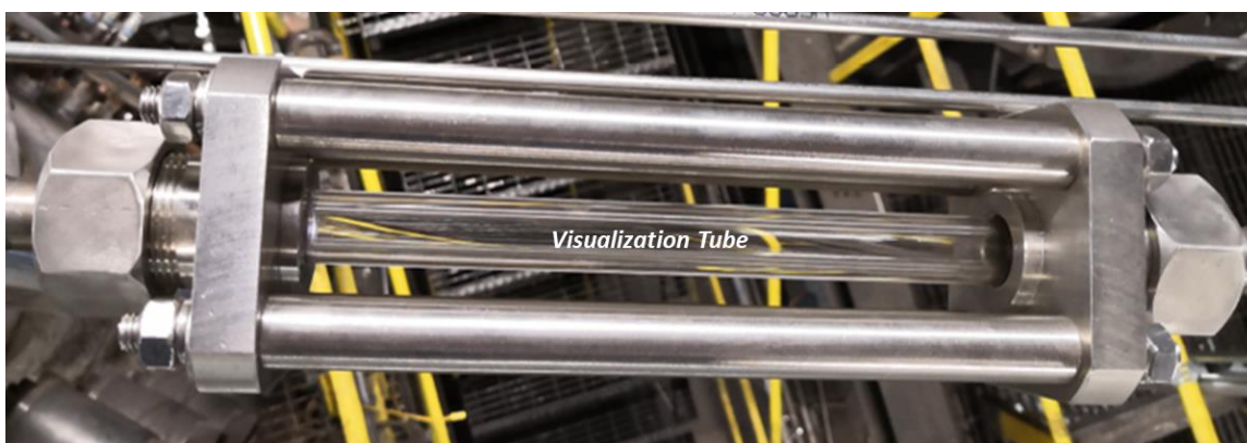
Figure 44. Visualization section for monitoring coal flow from the hopper to the reactor
