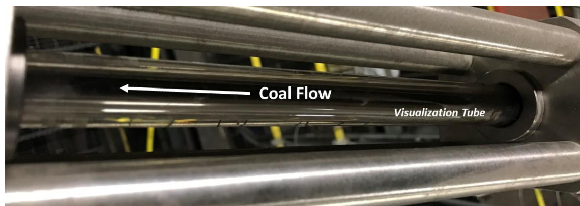
Figure 45. Visualization section with coal flowing from the hopper
