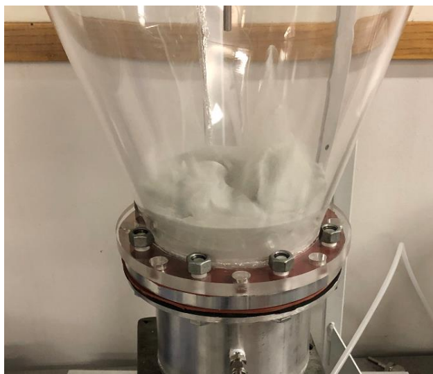
Figure 18. Fluidization of surrogate pulverized coal. The level of material in the photo is lower than during normal operation so that the fluidization can be seen.
