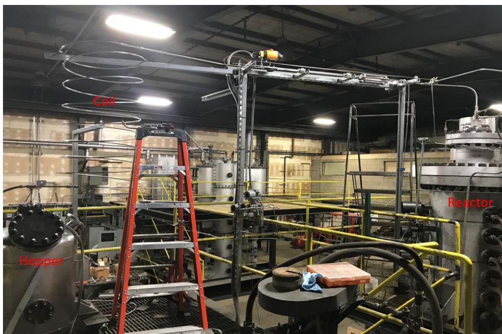
Figure 42. Integration of the dry feed system with the combustor showing the feeder hopper, coiled tubing, and EFPR
