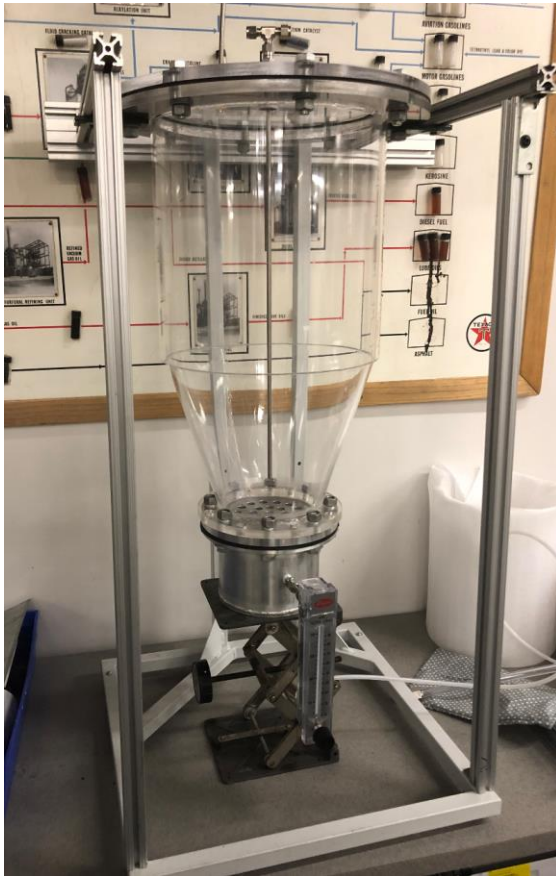
Bench-scale cold flow model of dry feed system hopper
