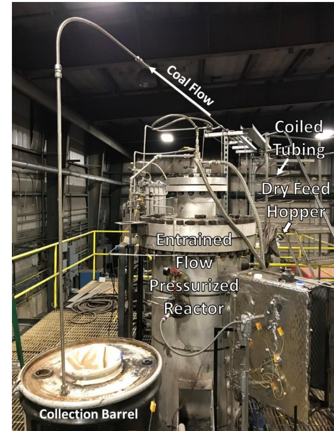
Non-reacting coal transport with the dry feed system
