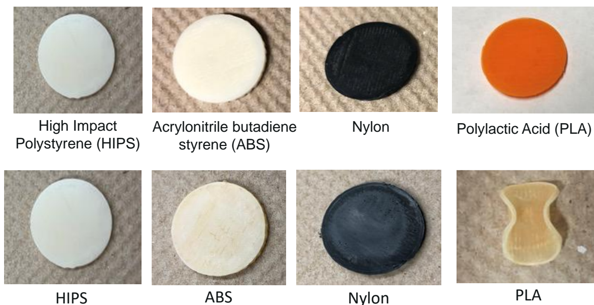
Figure 23. Polymer coupon before (top) and after exposure to CO 2 -rich amine solvent solution 6000 total hours (1000 h at room temperature + 5000 h at 60 °C except PLA which only after 1000 h at room temperature).
