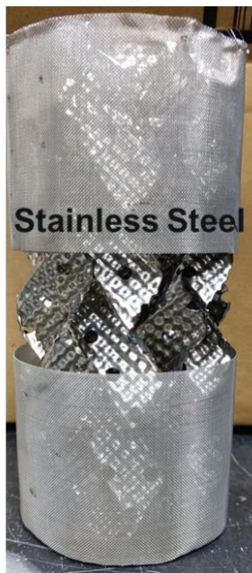
Figure 28. Stainless steel Mellapak 250Y packing material with 3" diameter.
