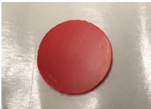
Figure 17. Polished ABS coupon used as the base for contact angle ( \theta ) measurements.
