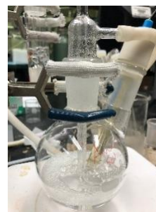
Figure 16. At 0.05wt.%, the solution produces relatively smaller, less stable bubbles, but similar CO 2 adsorption rates.
