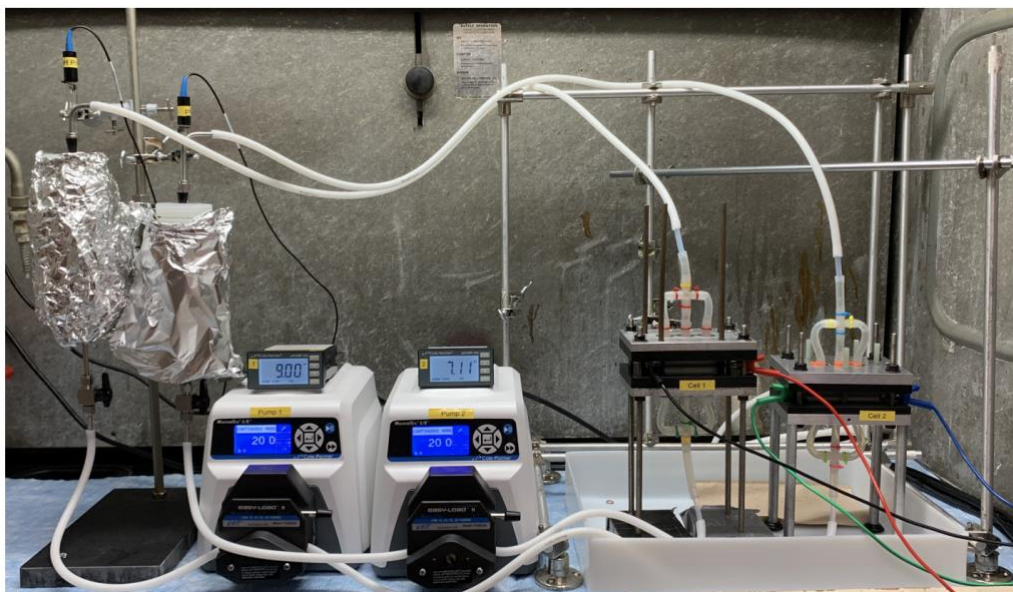
Figure 36. Flow through electrochemical cell for decomposing nitrosamines.
