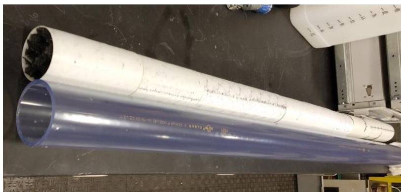
Figure 27. Dynamic packing produced by LLNL and used during long-term testing (Task 8)
