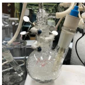
Figure 15. At 0.1wt.%, the solution produces larger and relatively more stable bubbles upon saturation with CO 2 .
