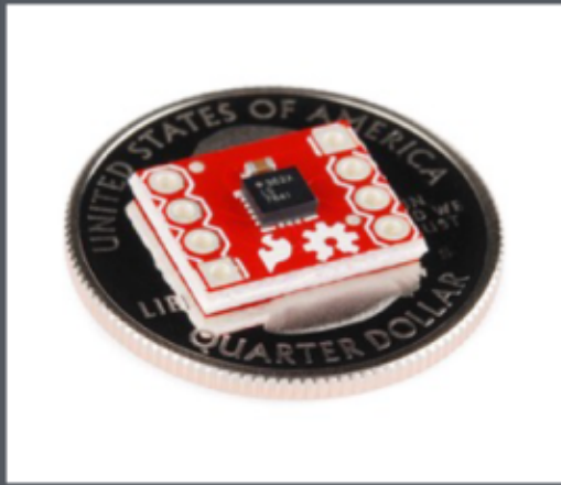
ADXL362 Triple-axis accelerometer Sensitivity : 1 mg/LSB Price $15 Source: Sparkfun
