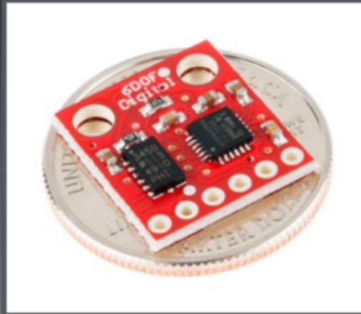
ITG3200/ADXL345 Inertial measurement unit Sensitivity : 4 mg/LSB Price $45 Source: Sparkfun
