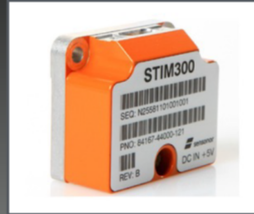
STIM300 Inertial measurement unit Sensitivity : 2 \mu g/LSB Price $15 Source: Sparkfun
