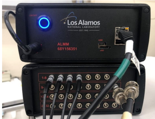
Figure 2.11 The ALMM data acquisition system used in the experimental setup. The four detectors are connected to channels 1-4 and the generator's source trigger is connected to channel 16.
