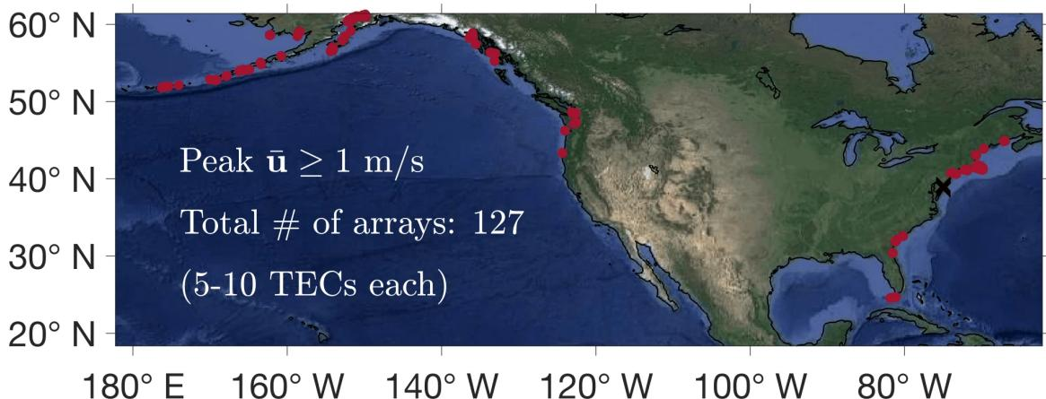
At each site, one TEC location is selected as the FI location. The rest of the sites are the MV measurement locations, at each of which we randomly sampled 500 timestamps out of the 2012 records. The tidal current records that start from these sampled timestamps were then extracted at a one-hour sampling rate. Record durations vary from 12 to 240 hours.
