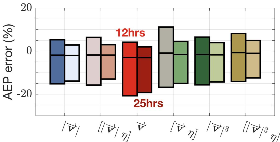
The variation of the AEP uncertainties based on the measurement period for 12 or 25 hour MV measurements are shown below. The results show a relatively steady mean error of -3%, suggesting that the strategy of combining a FI and a MV measurement is a viable option while also suggesting to some degree the underprediction of the available AEPs when applying our inferred framework.
