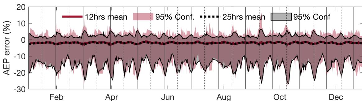
More interestingly, the temporal variation of the AEP errors shows a clear fluctuation with respect to spring/neap cycle. Specifically, the AEP errors reach to local extremes, when the MV measures neap tides (vertical gray lines). In contrast, the range of AEP errors is the smallest when measuring spring tides (in between gray lines).
