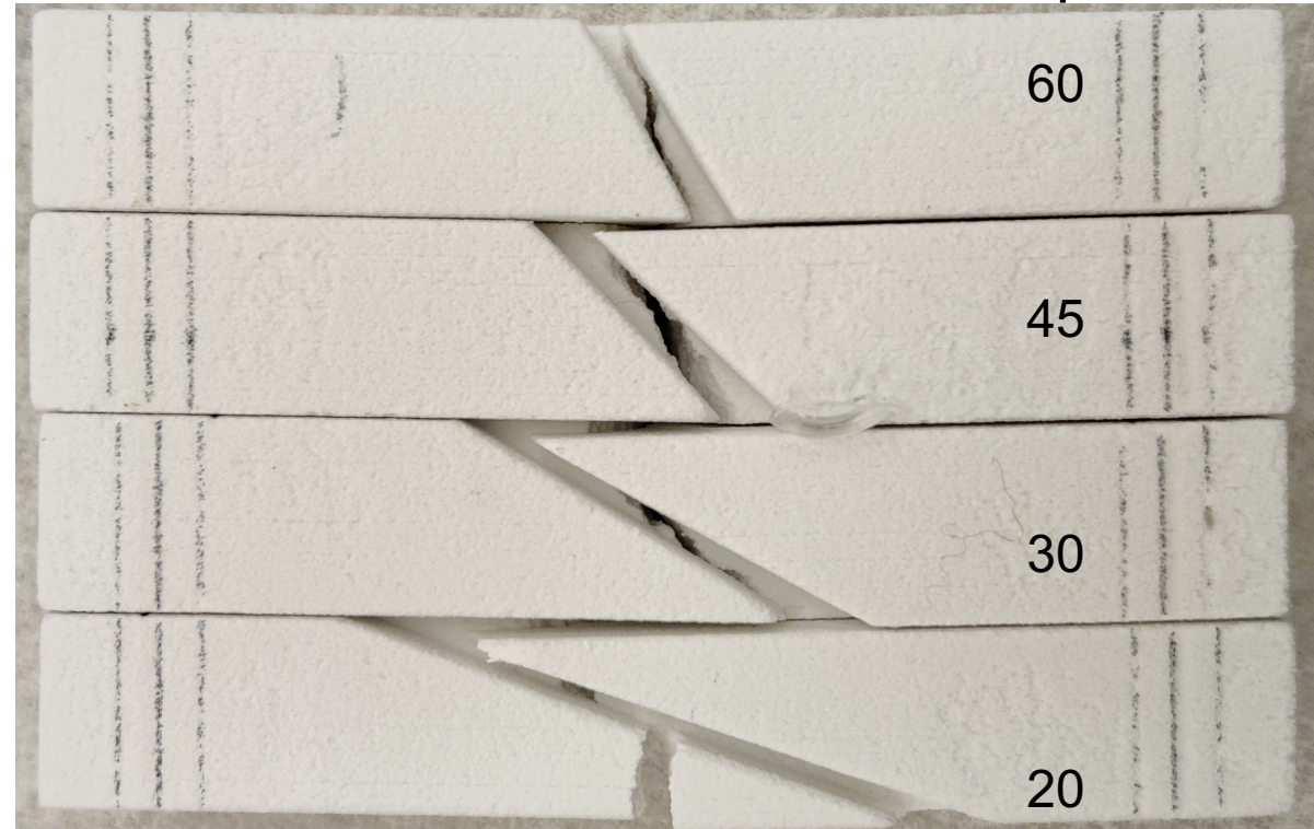
Bottom View of Cracked H Sample
