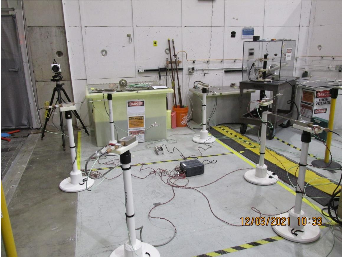
The Ddot signals were recorded on a six-channel Tektronix oscilloscope (MSO66B) at 1 TSps with 3 GHz bandwidth for a 10 us window, and the window was roughly centered in time on the arc (current) onset. A second oscilloscope (MS064) recorded current through the gap and voltage at the top electrode, also at 1 TSps with 3 GHz bandwidth. The first (Ddot) scope was triggered off the current on the second scope, and the scopes were time synchronized.
