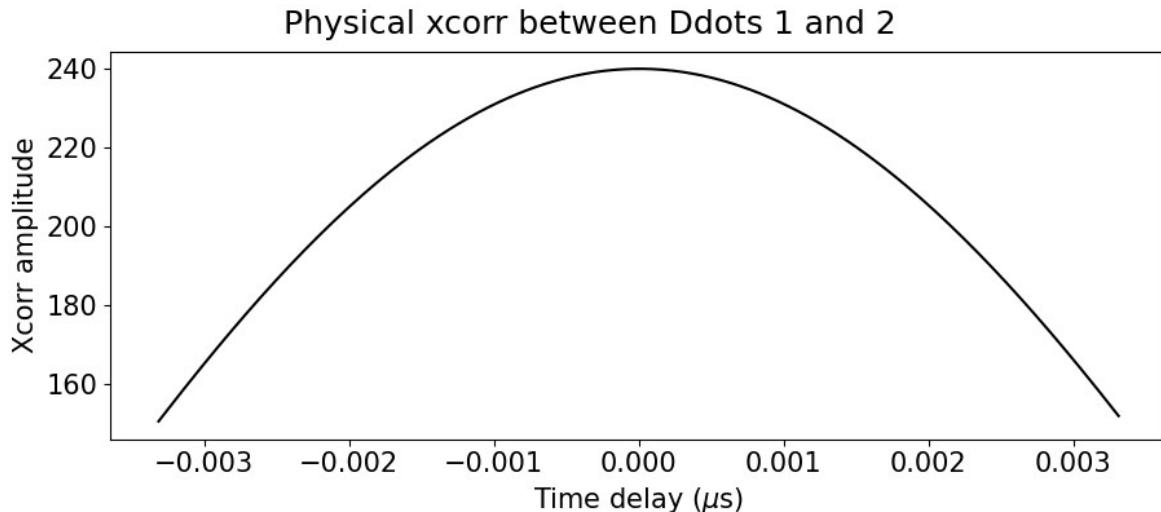
The "physical" cross correlation above is what is used to make the resulting radioimage. Note that for a point source, we would ideally like a sharp peak in the cross correlation. However, our source region was likely on the order of the spark gap size, so 100 mm, which was comparable to the size of the array with its 1-meter baselines. Hence our source appears to be very broad and fuzzy in the below 6-sensor radioimage.
