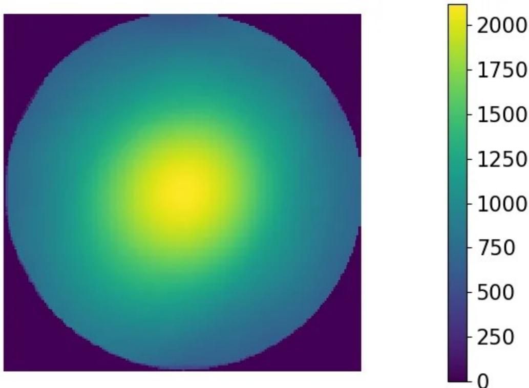
The below plot shows the same radioimage but without beamforming, clearly showing that the physical direction to the source was low on the horizon.
