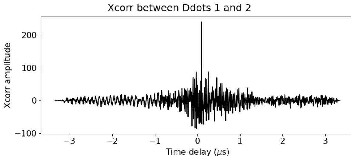
Because the spark gap is low on the "horizon" of the Ddot array, we used beamforming to center the source in the image plane. In the following plot, the peak of the cross correlation between Ddots 1 and 2 was centered at zero time delay. The other Ddot signals were similarly shifted in time with respect to Ddot 1 to perform beamformed radioimaging.
