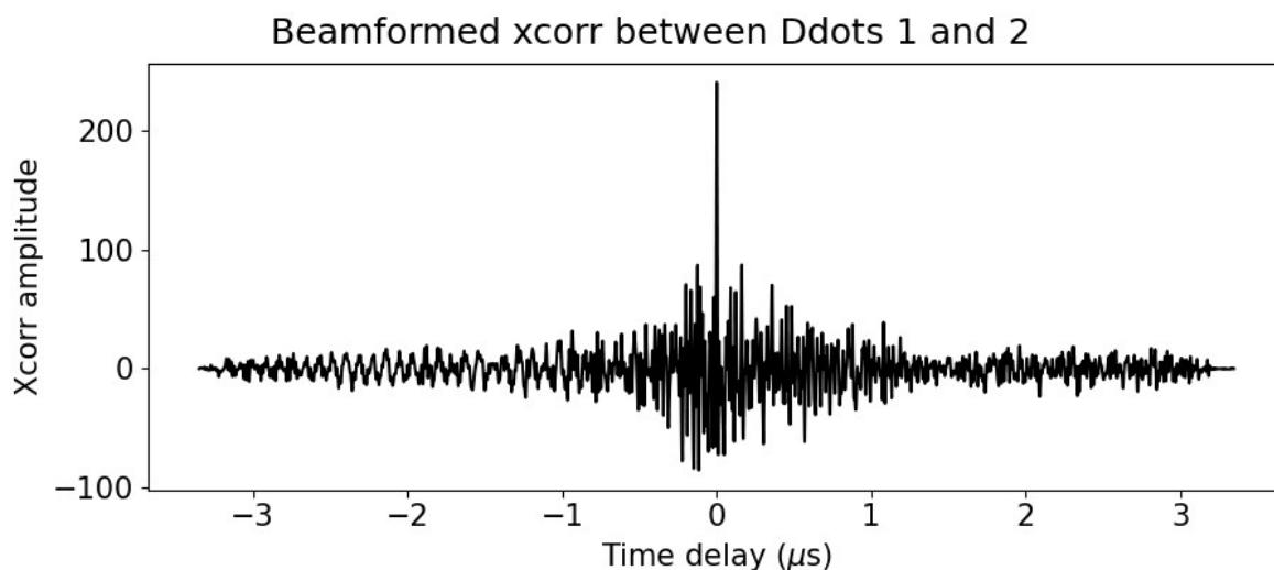
Not all the time delays shown on the above x-axes are "physical." That is, the distance between Ddots 1 and 2 is about 1 m, so that the longest light time of flight between the sensors is about 300 ns. In the below plot, the time delays (x-axis) are limited to values between  $-d/c$  to  $+d/c$ , where  $d$  is the baseline length and  $c$  is the speed of light.
