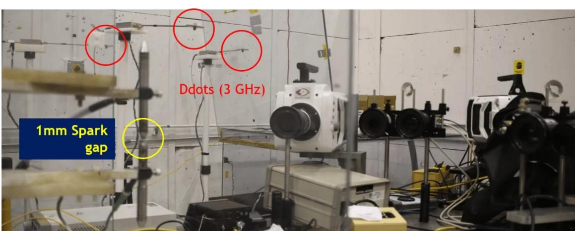
Several high speed cameras were used for both optical imaging and spectroscopy.
