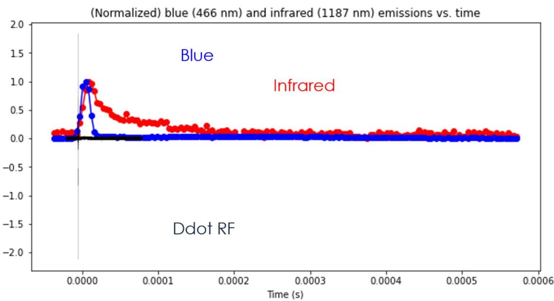
Note that the blue emissions, presumably due to corona discharge (cold plasma) turn on and off quickly compared to the IR emissions, presumably due to the (thermal) arc discharge.
