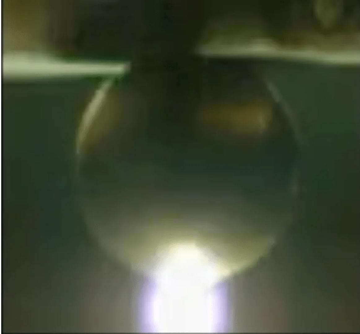
However, at 440 kfps (2.26 us / frame), one frame of streamer activity preceded the arc onset. Note that the 711 was zoomed in on the very bottom of the top (positive voltage) electrode. The streamers are visible as blue filaments in the frame prior to saturation.
