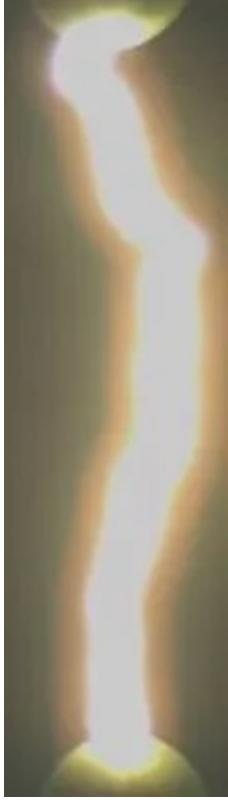
Any precursor activity (e.g., corona discharge) prior to arc onset was not visible at this timescale.
