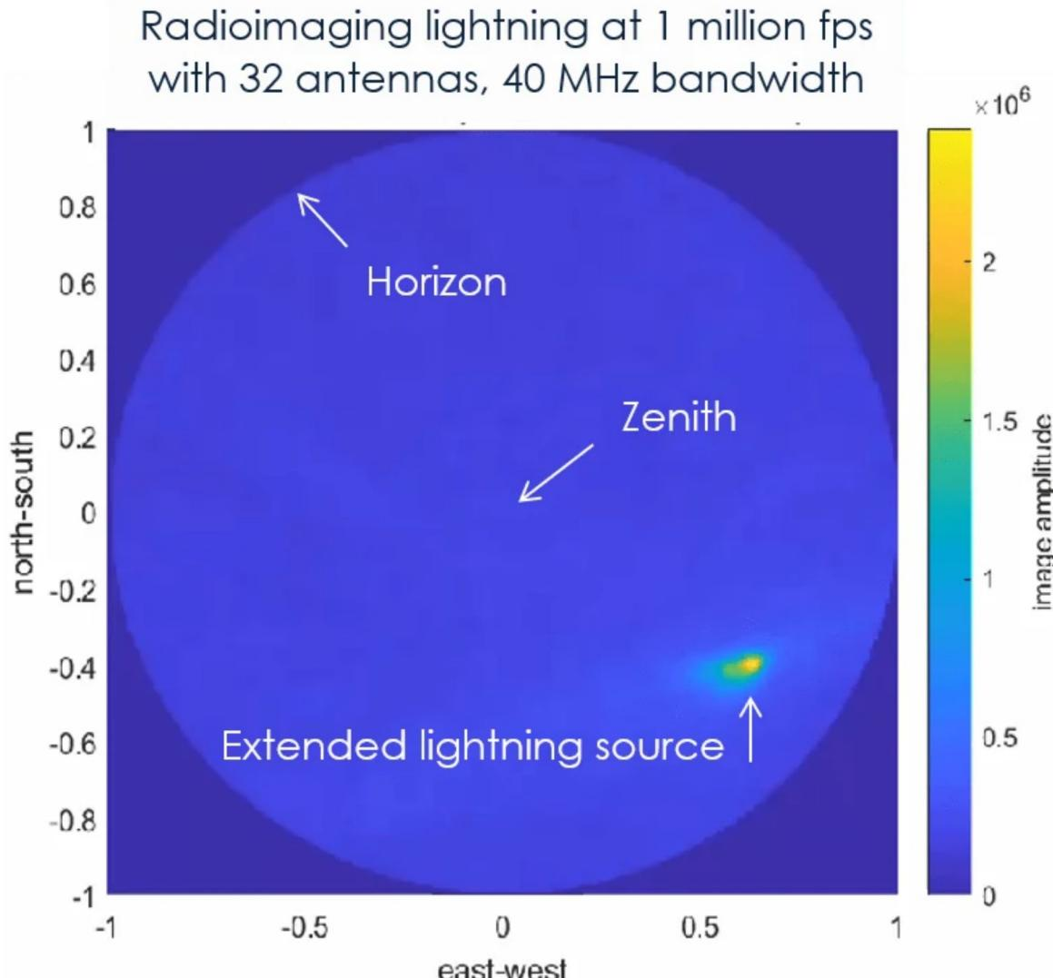
Radioimaging is a relatively new technique for studying lightning, and is an emerging diagnostic for high voltage systems at Sandia National Labs. We have previously shown that electrical breakdown at lab scales emits copious amounts of broadband RF emissions from DC up to at least 3 GHz. In the below figure, the top plot shows the time-domain RF signal associated with an arc bridging a 142-mm spark gap, and the bottom plot shows the spectrogram on the same timescale.
