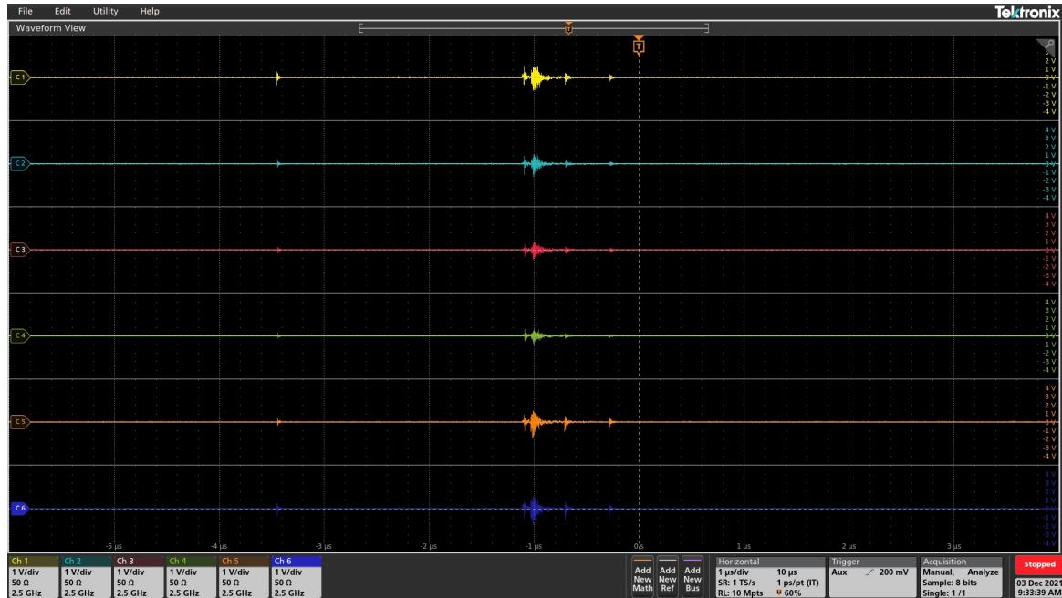
The precursor RF activity is shown on a shorter timescale (100 ns across) below, clearly showing different arrival times at the six Ddots. The top trace comes from the closest Ddot to the spark gap (placed 1 m away from the spark gap), and the following traces come from Ddots placed counter-clockwise with respect to the first Ddot.
