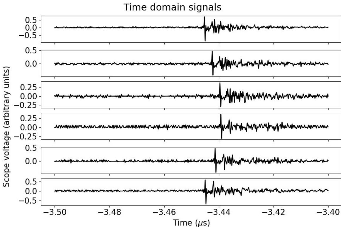
The above signals are Fourier transformed and shown in the next plot. Note the broadband emissions from DC to about 3 GHz.
