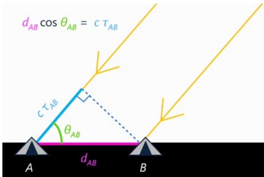
The arrival angles can be mapped into sky coordinates to denote the direction from the sensor array to the radiating source(s), as shown in the below figure.
