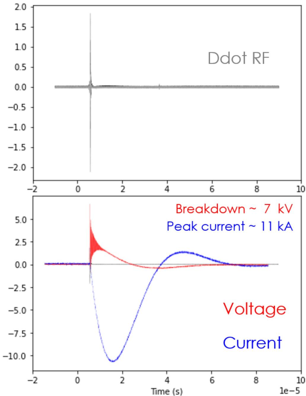
The current through the hot arc lasted nearly 100  $\mu$ s, while the RF was incredibly prompt in comparison. The same data is shown below on a shorter time scale, showing a burst of RF activity nearly coincident with the arc current onset (also note the voltage collapse). There were also RF emissions prior to arc onset, presumably due to corona discharge.
