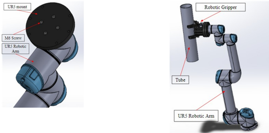
Figure 19. UR5 mount for the Robotic Gripper
