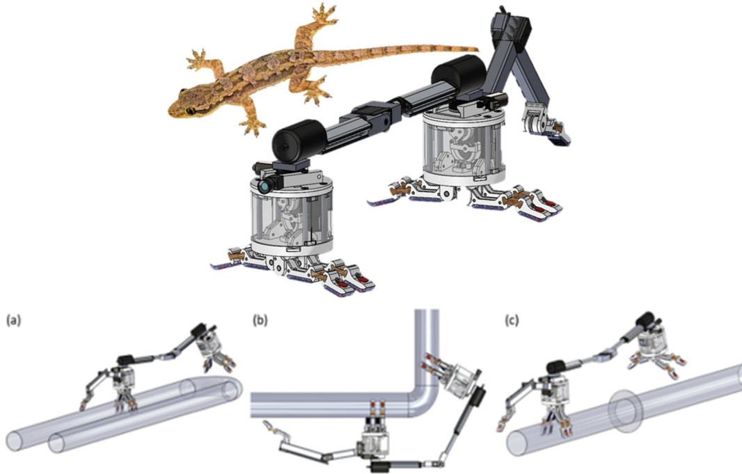
Figure 50. Conceptual design of the Lizard Inspired Tube Inspection Robot.
