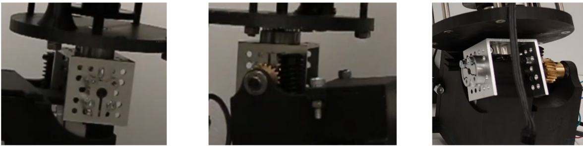
Figure 56. The front and back side of the U-bracket in the first design of gearbox B.
