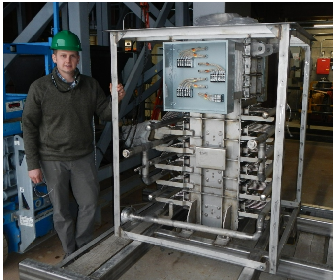
100 kW particle-to-sCO 2 heat exchanger
