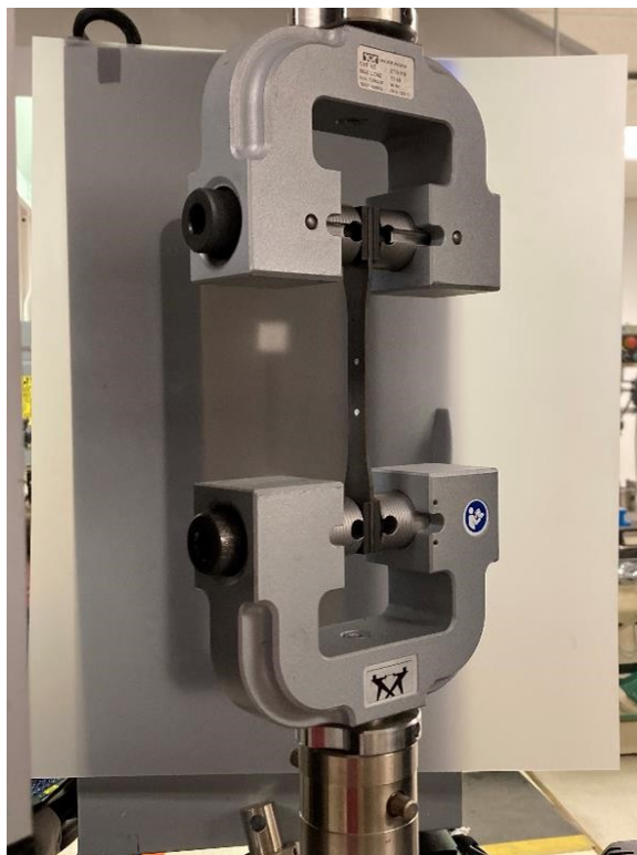
Figure I.1.1.4. Picture of a Fe 4 N/epoxy composite undergoing tensile testing at NREL.
