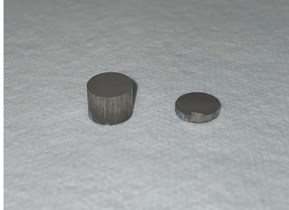
Figure I.1.1.5. 75.3 vol.% \text{Fe}_4\text{N} in epoxy SMC. The shorter cylinder was cut using a diamond saw for VSM analysis.
