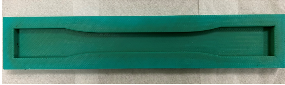
Figure I.1.1.1. Silicone mold for the fabrication of dog bone test structures.
