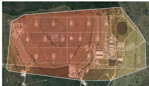
Figure 3-7. Contour plots displaying average subsidence rates at Big Hill over three different time periods identified from Figure 3-6
