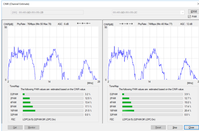
Fig. 7. Capture from BlueChip's tool showing CINR over 2 to 28 MHz spectrum with corresponding bit loading and data rates.
