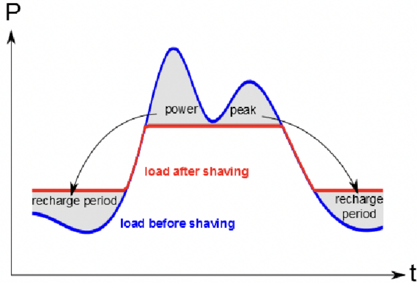
Figure 6. Example of peak shaving in a power load schedule – y axis power, x axis time
