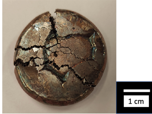
Figure 2.6 Fe-6.5Si wt% sample failing after only 5% reduction during hot rolling.
