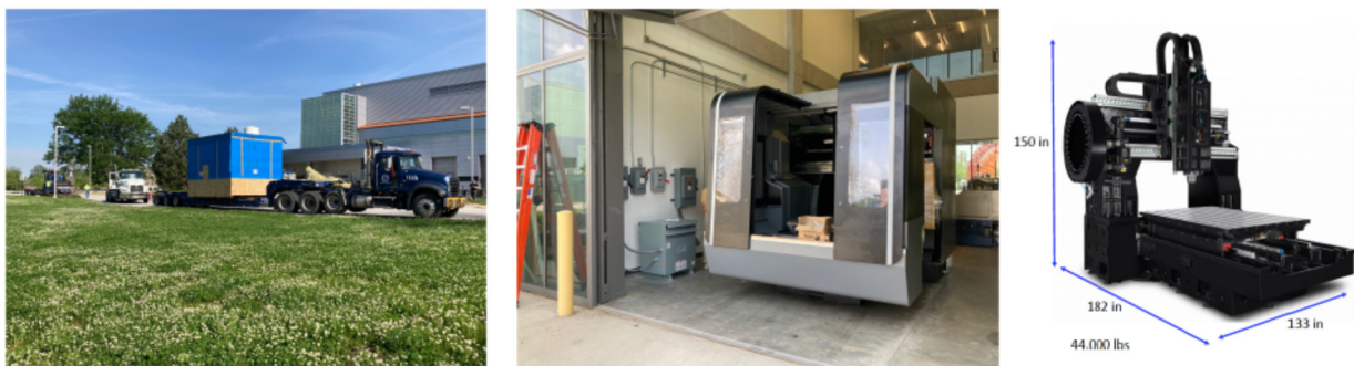
Figure 4.3 Base Machine for 150 mm wide strip – Linear configuration. The picture on the right is a rendering of the physical process configuration layout within the machine.
