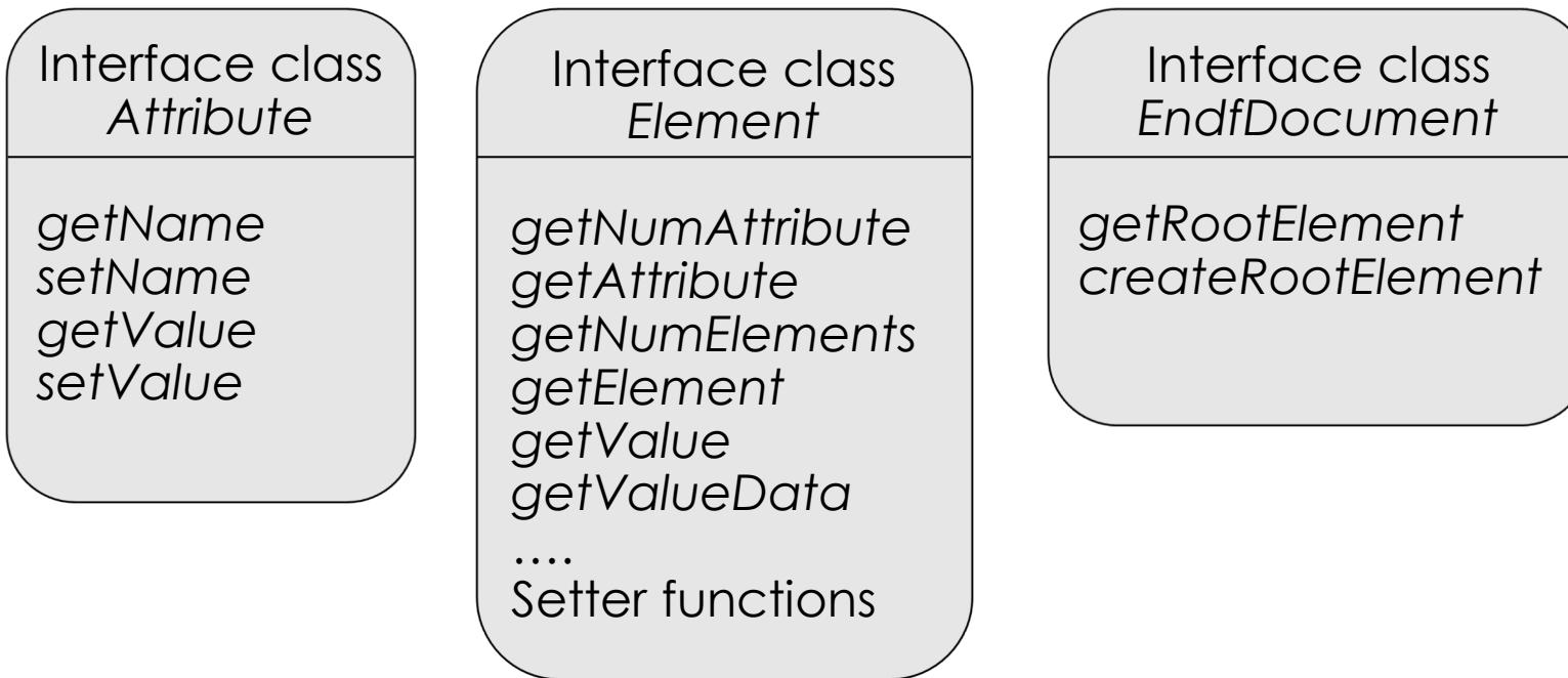
Based on pugixml. This is a layer on top of the actual XML DOM reader to allow easy switch to different reader if needed.
