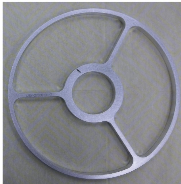
Fig. 8. Photograph of an aluminum spacer used to introduce voids in the lead moderators of the Zeus HEU and IEU cores.
