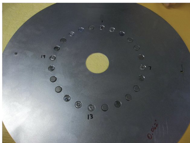
Fig. 6. Photograph of activation and fission foils loaded on a sample plate for irradiation in a Zeus HEU core.
