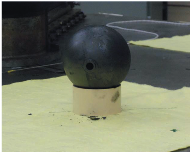
Fig. 11. Flattop HEU core.
