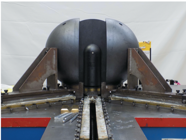
Fig. 6. Flattop pedestal and HEU core seated in stationary reflector.
