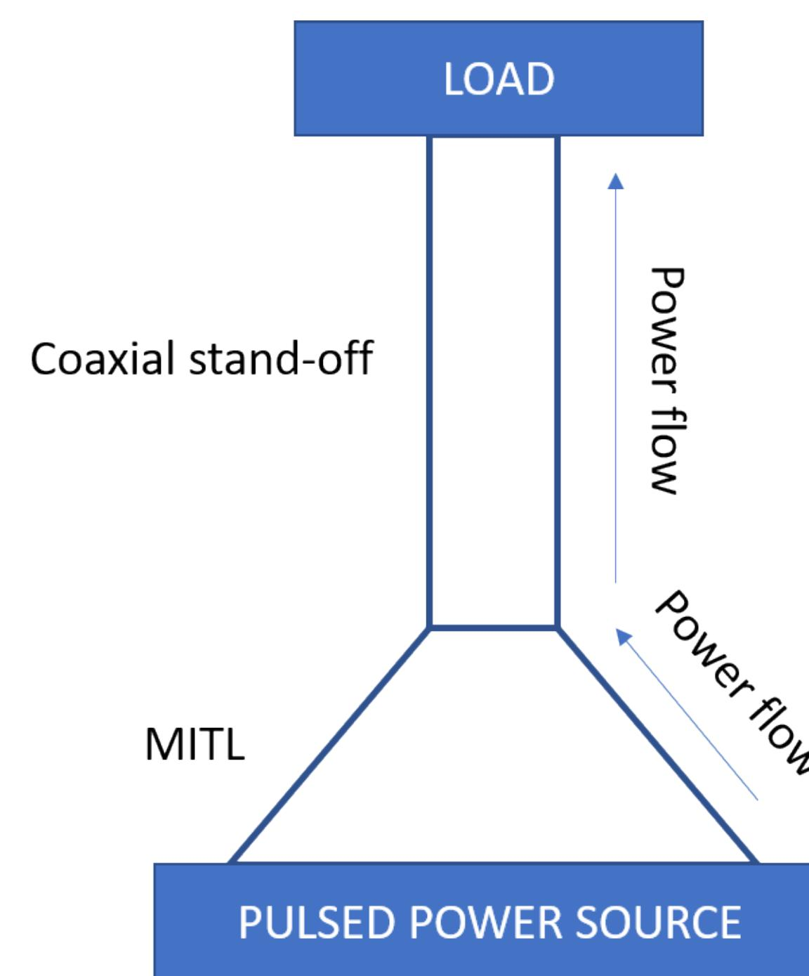
The transition from a conical to coaxial transmission line requires
