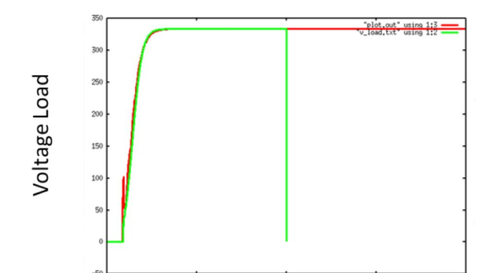
Initial results show expected behavior for voltage at the load that agrees with lumped element circuit models.
