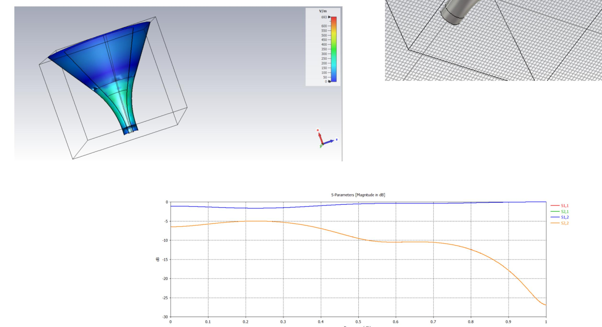
A circular profile is applied at the conical to coaxial transition that reduces the electric field but maintains transmission of power over the frequency band from 0.1 GHz to 1 GHz
