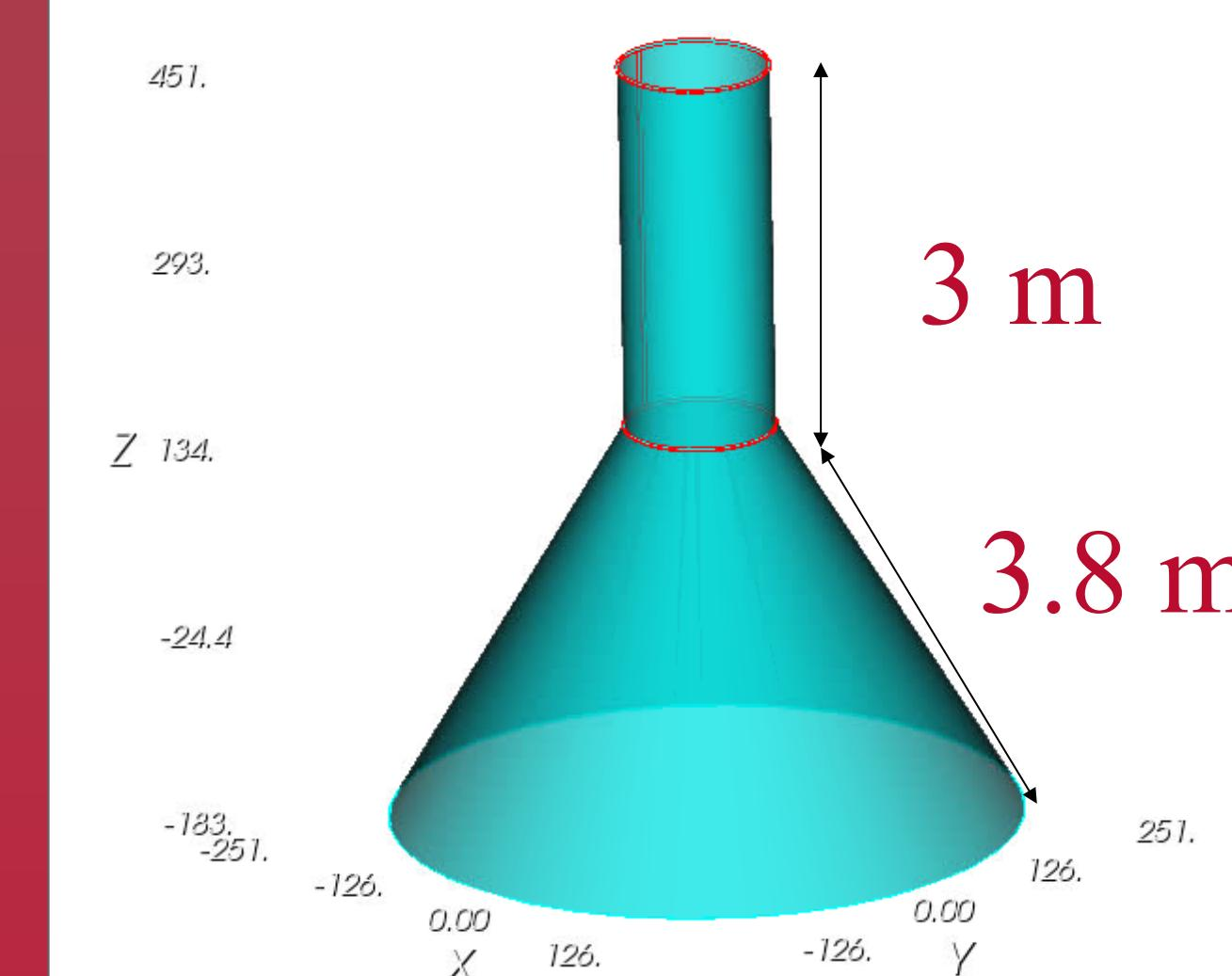
A 1 degree wedge of the entire simulation domain still results in ~9.5 million elements with a 1 mm mesh resolution. The conical and coaxial lines are designed to have a  $0.3 \Omega$  impedance leading to roughly 2-3 mm gap sizes.
