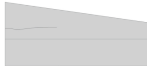
(a) Crack path in tapered specimen predicted by FRANC3D
